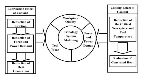
Fig. 1. Primary effects of lubrication and cooling in the machining process after Brinksmeier et al. (1999)
