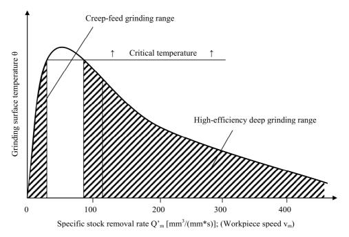
Fig. 5. Surface temperature trend in HEDG after Tawakoli (1993)
