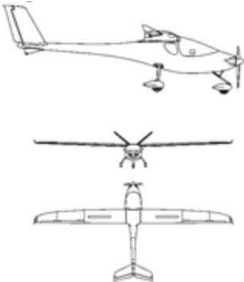
Fig. 1.6 Scheme of the Bye Aerospace eFlyer 4
