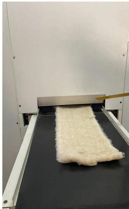
Figure 2.17 – Needle punching of fibers
