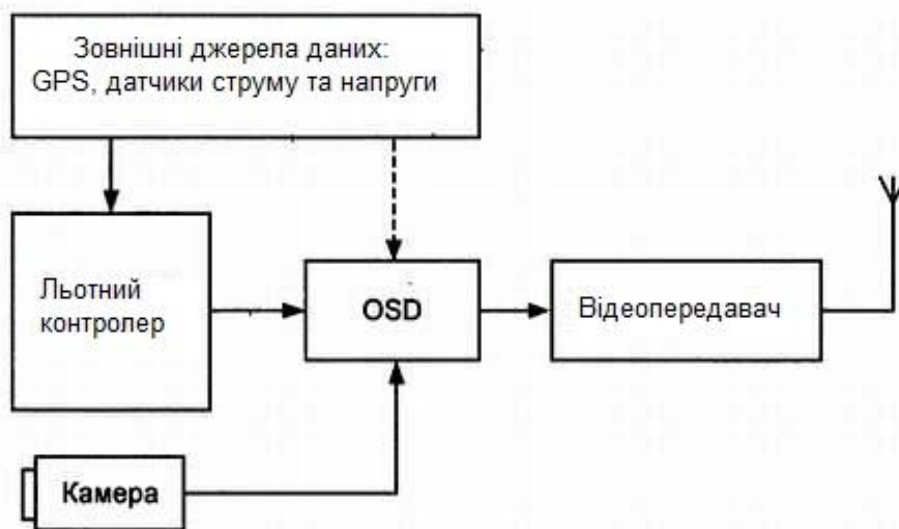
Figure 3.16 - Block diagram of telemetry application with OSD.
