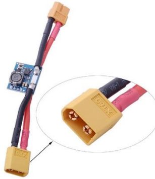
Figure 3.6 - Power module APM BEC 3A XT60 plug
