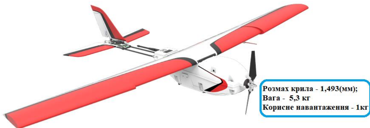
Fig. 1. 2 - Lancaster UAV – for scientific research work.
