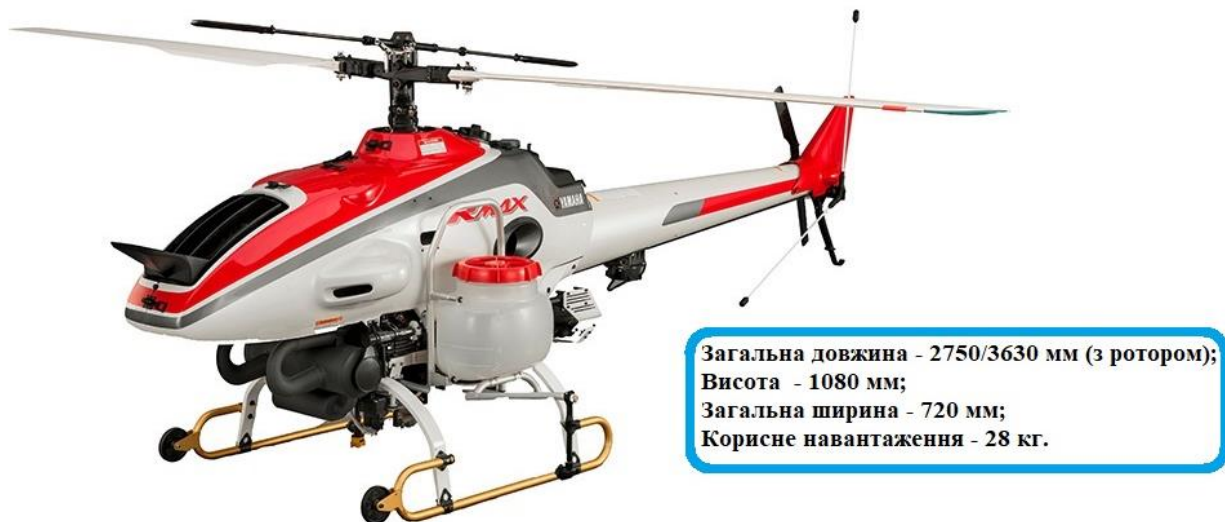
Figure 1.1 - Yamaha RMAX UAV - for field spraying.
