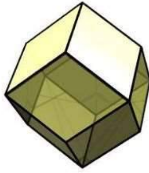
Figure 2.17 – The range of changes in the vector of the kinetic moment H for a minimum-excess pyramid scheme
