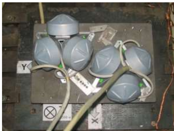
Figure 2.19 – Placement scheme of six EFMs
