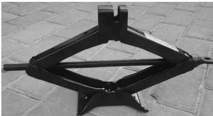
Fig. 1.6. Jack with lever and screw mechanisms
