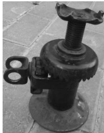
Fig. 1.4. Jacks with mechanical transfer: a – worm; b – bevel
