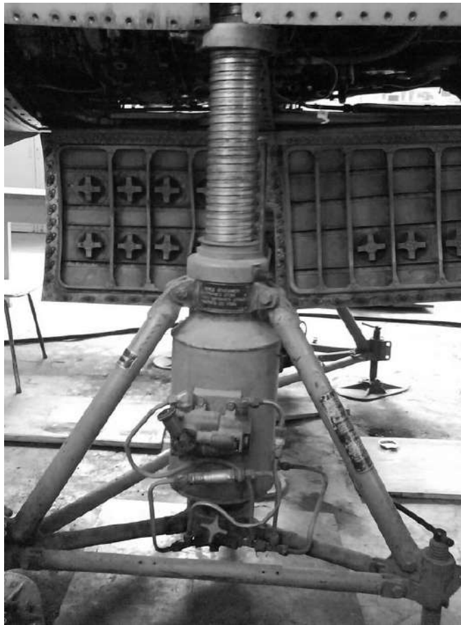
Fig. 1.5. Screw jacks with a hydromotor
