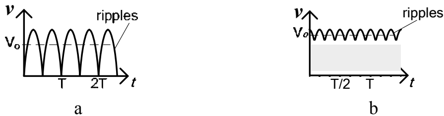
Fig. 2.3 – The waveform of DC generators: with 2-segment commutator (a); for multi-loop armature and multi-segment commutator (b)
