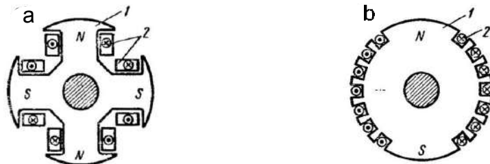
Fig. 4.3 – The rotors of a synchronous machine: salient pole rotor (a); cylindrical rotor (b)
