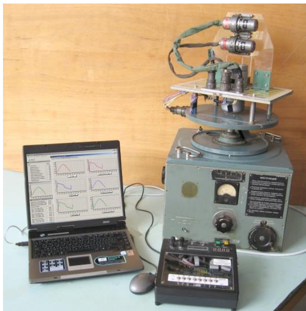
Fig. 5. General view of the stand for the study of sensors in the yaw channel
