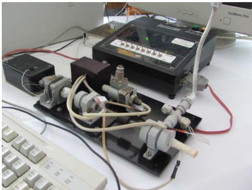
Fig. 1. Appearance of experimental mock-up model based on the small-sized vortex energy separator
