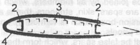
Fig. 3.32. Monoblock wing with two false spars
