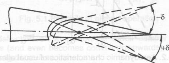
Fig. 5.4. Aileron with lowered rotation axis
