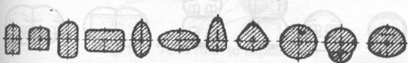
Fig. 8.1. Shapes of fuselage cross-sections
