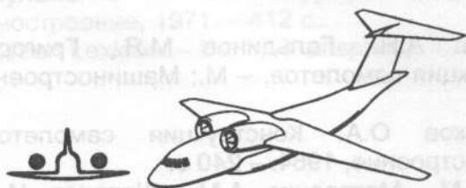
Fig. 12.9. Arrangement of engines above the wing
