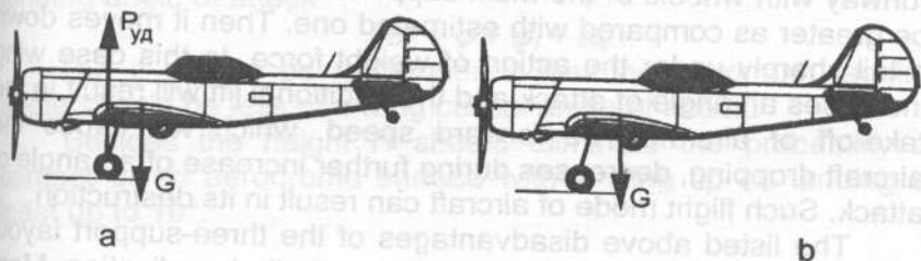
Fig. 9.2. Possibility of periodic bouncing of aircraft after landing.
