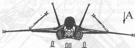
Fig. 3.50. Tilting outer panels
