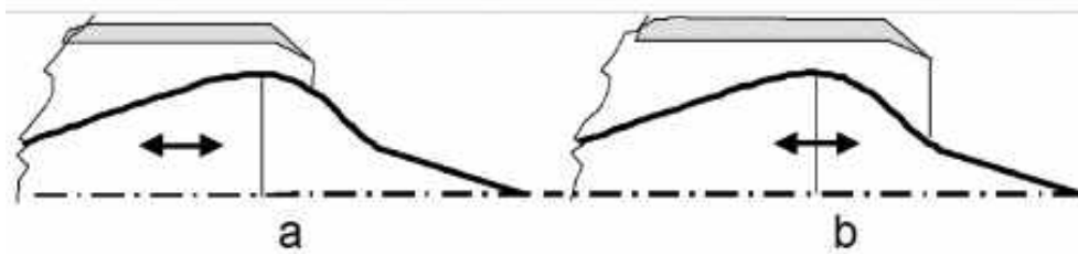
Figure 2.12 – Nozzle with central body: a – with external expansion; b – combined
