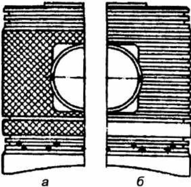
Figure 12 – Pistons: a – intake piston; b – exhaust piston
