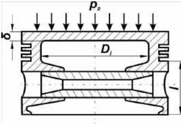
Figure 16 – Illustration to strength analysis
