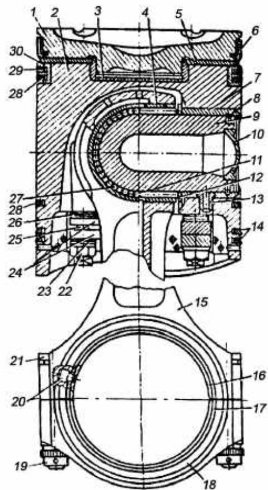
Figure 11 – Piston and connecting rod of 6TD RE
