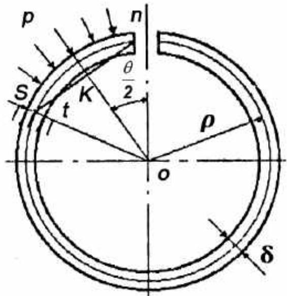
Figure 21 – Illustration to strength analysis of piston ring
