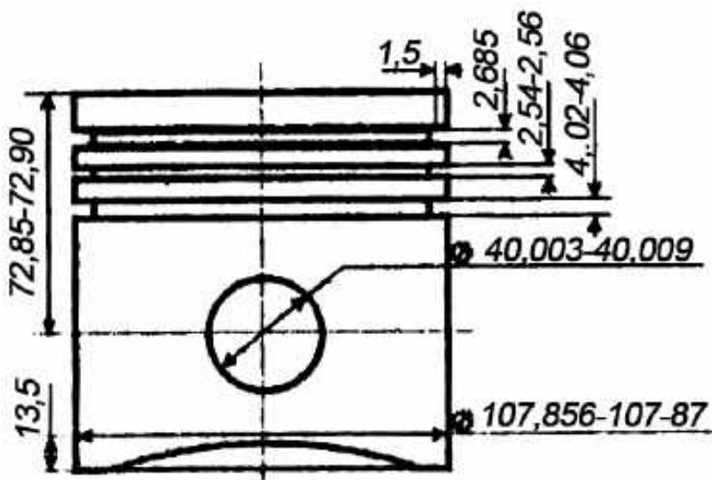
Figure 5 – Sizes of piston by ALKAN
