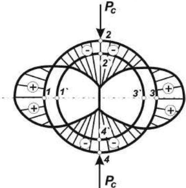
Figure 18 – Diagram of stresses in the piston pin at ovalized state
