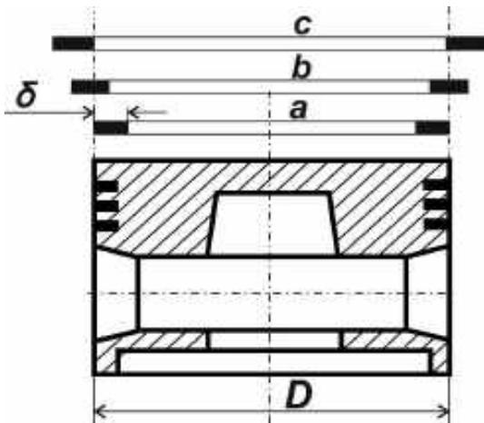
Figure 20 – The sizes of the piston ring: a –working state;  $\rho'' = R - \frac{\delta}{2}$ ; b – standalone state;  $\rho = R$ ; c – when fitting the piston,  $\rho'' = R + \frac{\delta}{2}$
