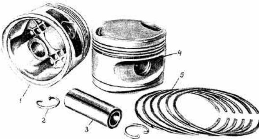
Figure 9 – Piston of ASH-82 RE
