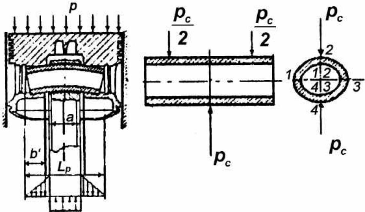
Figure 17 – Illustration to strength analysis of the piston pin
