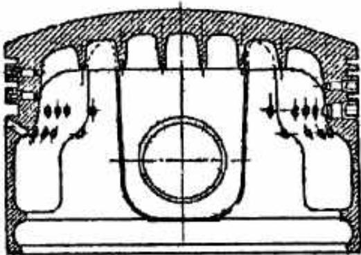
Figure 6 – Piston of V-type AM-38 reciprocating engine
