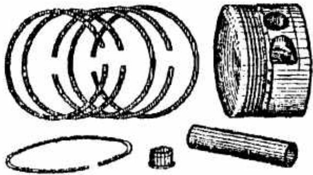
Figure 7 –Parts of AM-38 piston unit
