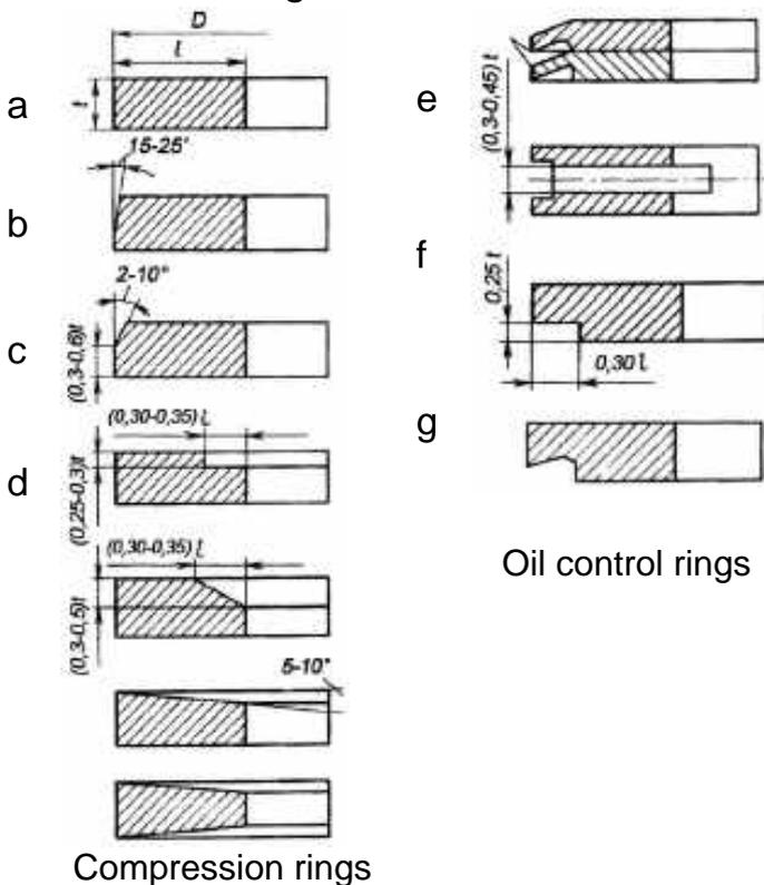
Figure 2 – Profile of compression and oil control rings
