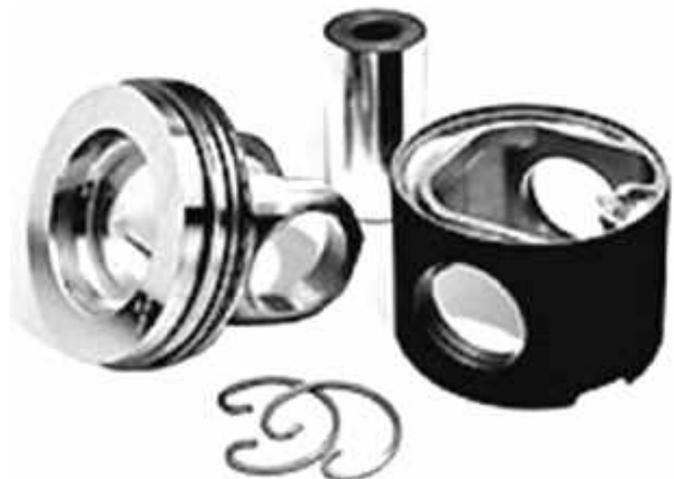
Figure 15 – Piston of VOLVO D12/D13
