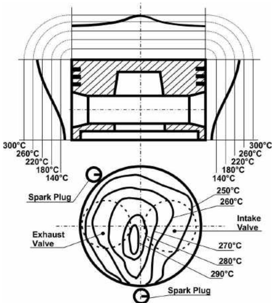
Figure 1 –Temperature distribution on piston surface
