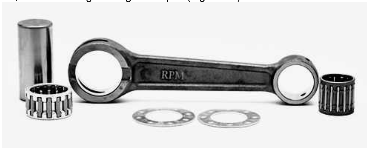
Figure 13 – Connecting rod of the ROTAX-582 with the pin and the needle sleeve bearing
