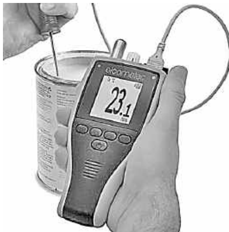
Figure 6.3 – Electronic dewpoint meter with optional liquid probe
