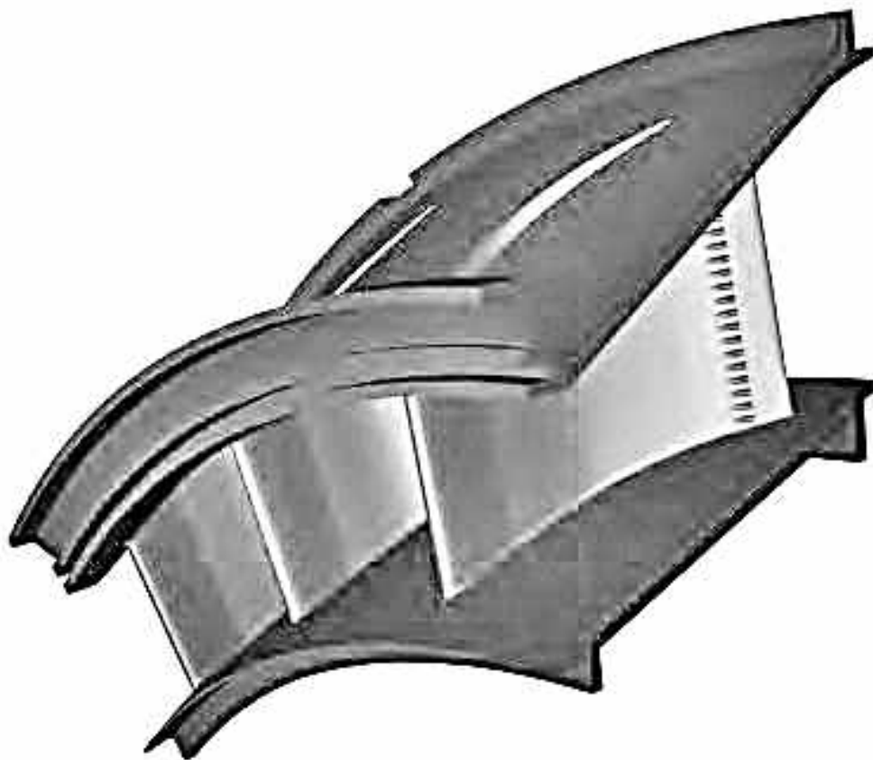
Figure 5.11 – Sector of the turbine II stage guide vanes (solid model)
