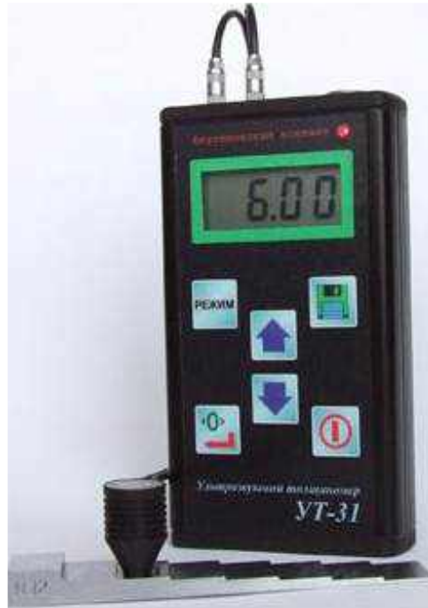
Fig. 7.15. Ultrasonic thickness measuring device YT-31
