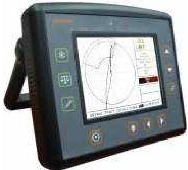
Fig. 7.11. Low-frequency ultrasonic defectoscope УД2Н-ПМ
