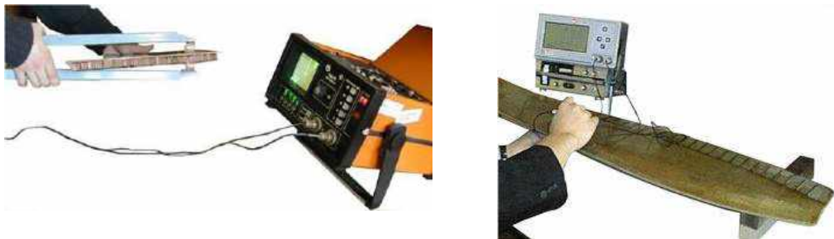
Fig. 7.9. Inspection of metal and non-metal adhesive honeycomb structures
