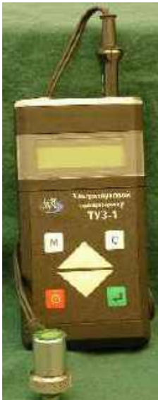
Fig. 7.14. Ultrasonic thickness measuring device TY3-1
