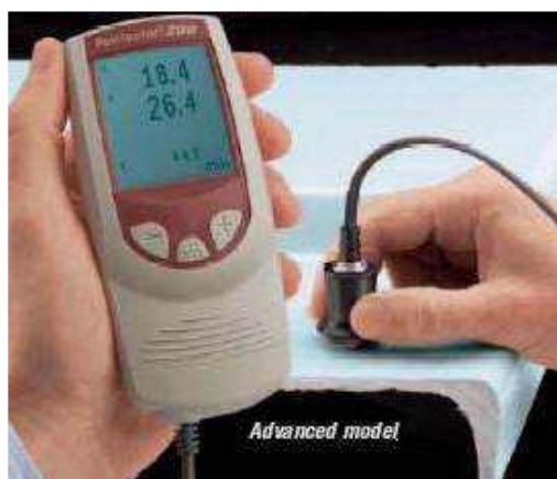
Fig. 12.2. Ultrasonic coatings thickness measuring device PosiTector 200
