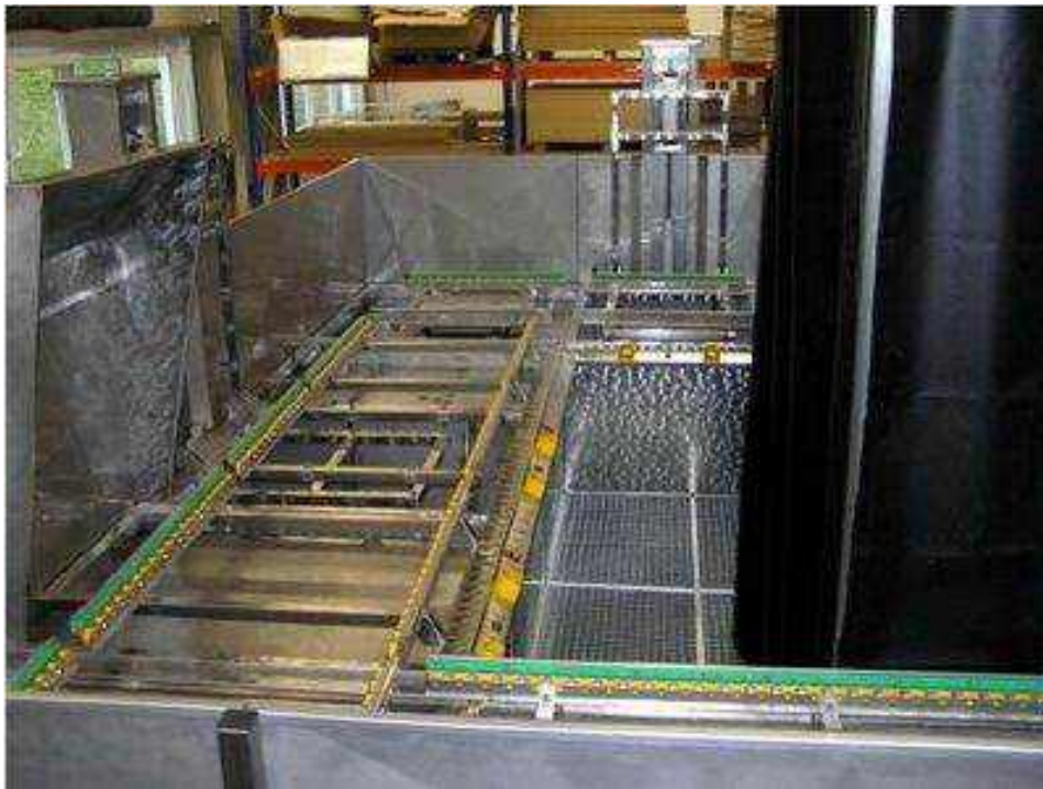
Fig. 6.5. Mechanized line with transport system of multi-roller conveyor track and mechanisms for articles lifting and dropping to a bath with reagents
