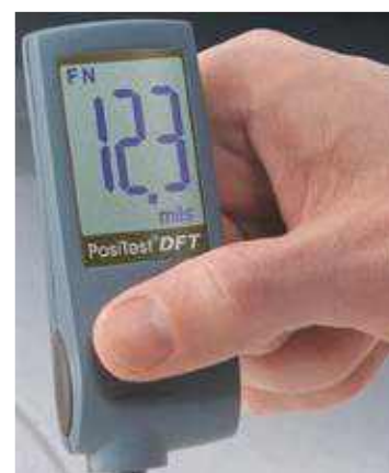
Fig. 12.4. Coatings thickness measuring device PosiTest DFT
