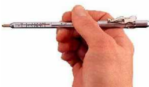
Fig. 12.5. Magnetic thickness measuring device PosiPen
