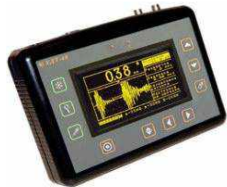
Fig. 7.16. High precision thickness measuring device with A-scan УДТ-40
