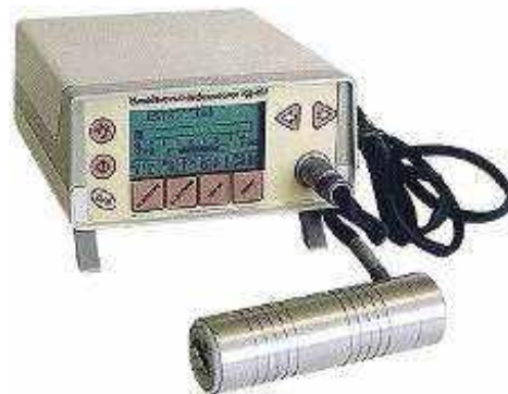
Fig. 7.26. Impedance defectoscope ИД-401
