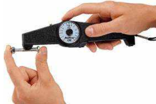
Fig. 12.6. Magnetic device for coatings thickness measuring Positest F/G
