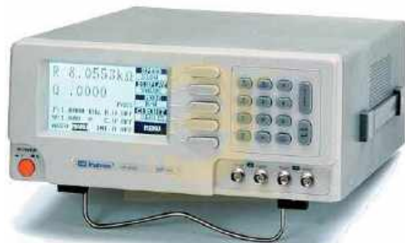
Fig. 8.3. RLC measuring device LCR-800 (by GW Instek manufacturer)
