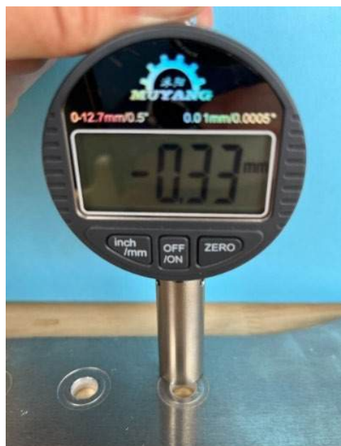
Fig. 7. Measuring the depth of the annular groove
