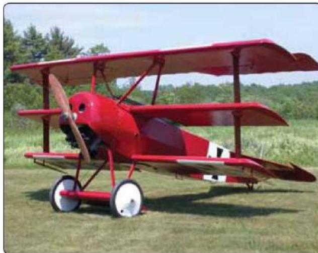
Figure 6.14 – Rigid steel landing gear is used on many early aircraft
