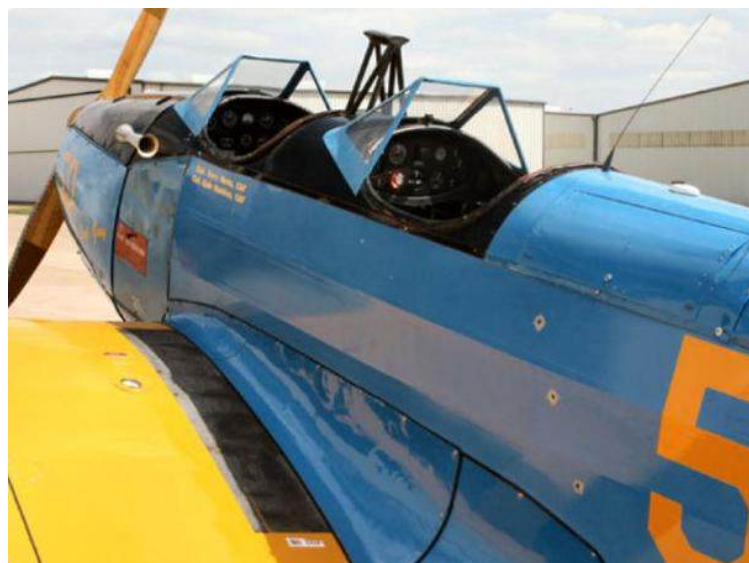
Figure 3.11 – Wing root fairings smooth airflow and hide wing attach fittings
