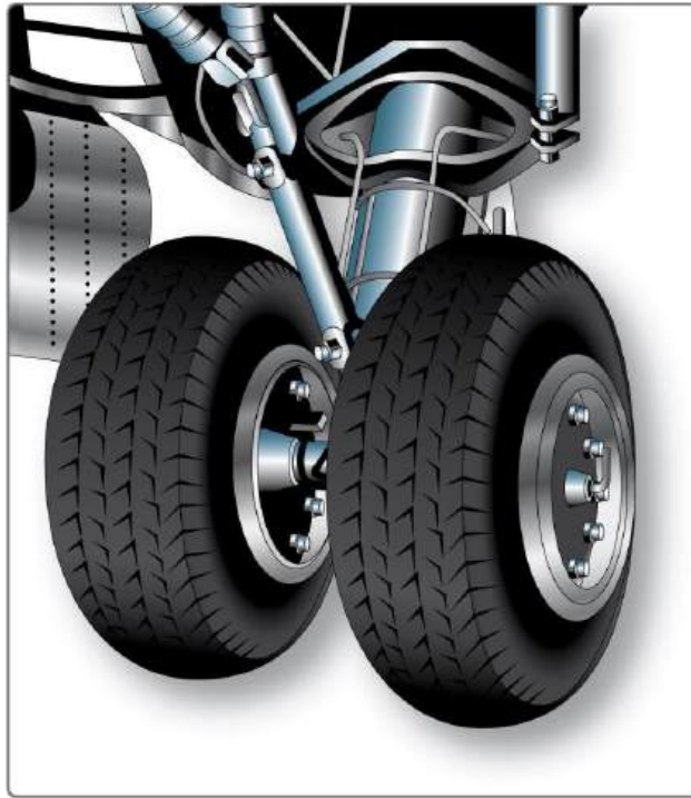
Figure 6.8 – Dual main gear of a tricycle-type landing gear
