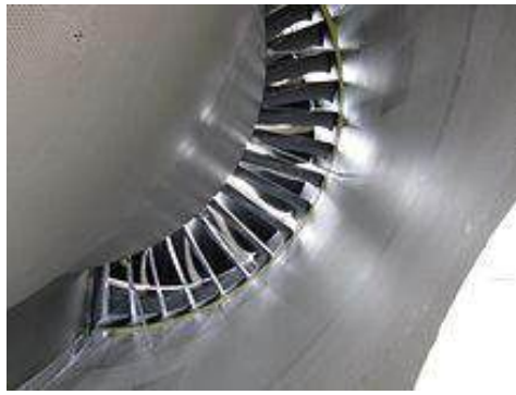
Figure 5.3 – View into the outer (propelling or "cold") nozzle of a GEnx-2B turbofan engine
