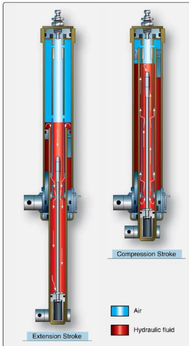
Figure 6.23 – Fluid flow during shock strut operation is controlled by the taper of the metering pin in the shock strut orifice
