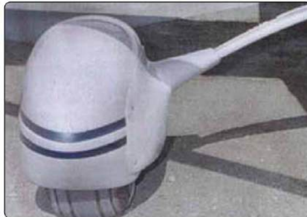
Figure 6.11 – Wheel fairings, or pants, and low profile struts reduce parasite drag on fixed gear aircraft
