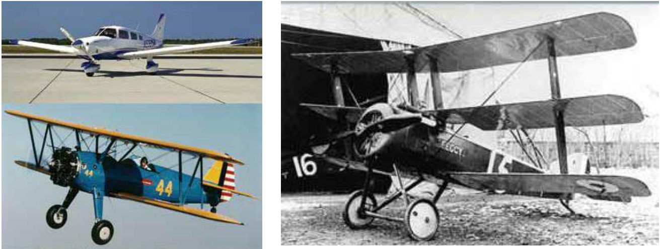
Figure 2.2 – A monoplane (top), biplane (middle), and tri-wing aircraft (bottom).
