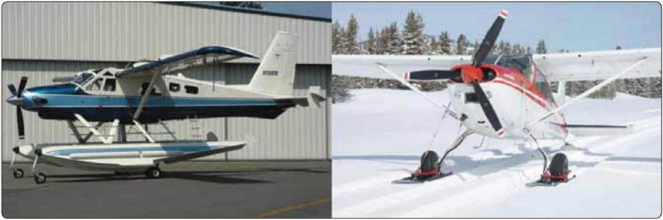
Figure 6.2 – An amphibious aircraft with retractable wheels (left) and an aircraft with retractable skis (right)
