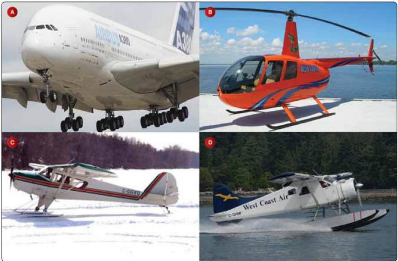
Figure 6.1 – Basic landing gear types include those with wheels (a), skids (b), skis (c), and floats or pontoons (d)
