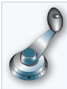
Figure 6.7 – A nose wheel steering tiller located on the flight deck
