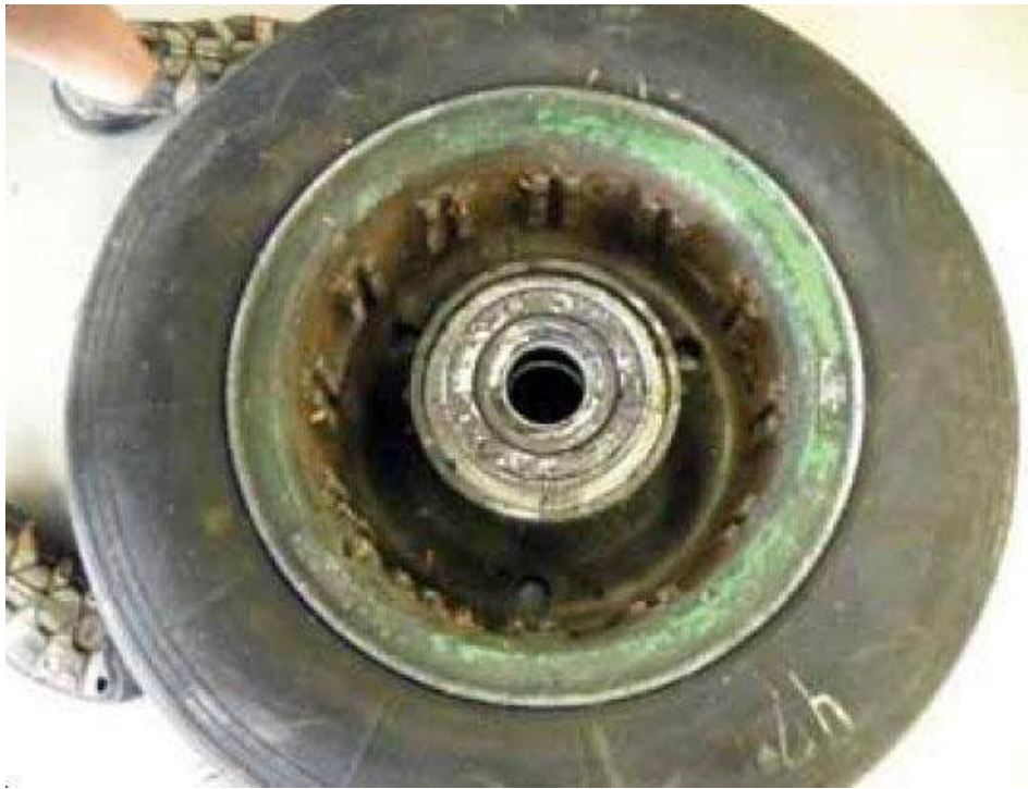
Figure 16.27 – Keys on the inner wheel half of an aircraft wheel used to engage and rotate the rotors of a disc brake
