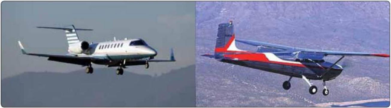
Figure 6.6 – Tricycle-type landing gear with dual main wheels on a Learjet (left) and a Cessna 172, also with tricycle gear (right)
