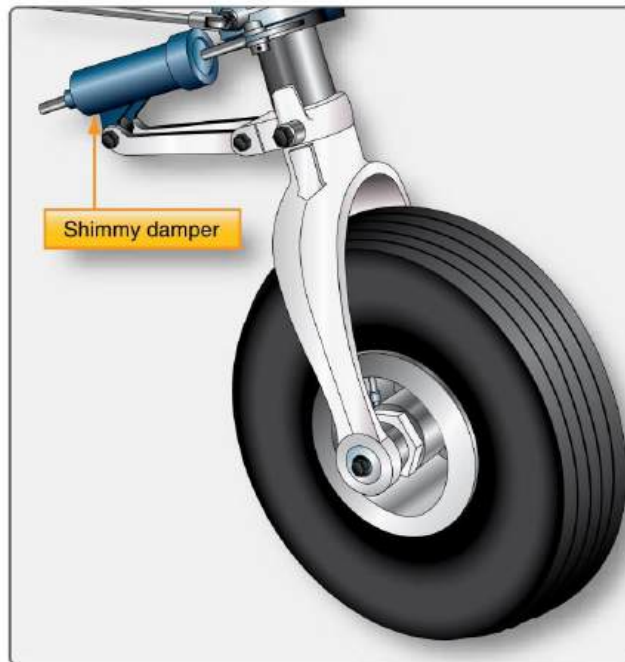
Figure 6.21 – A shimmy damper helps control oscillations of the nose gear
