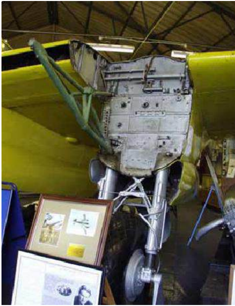
Figure 3.19 – An engine nacelle firewall
