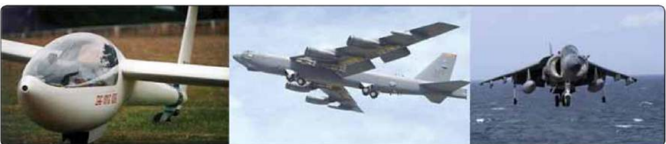
Figure 6.5 – Tandem landing gear along the longitudinal axis of the aircraft permits the use of flexible wings on sailplanes (left) and select military aircraft like the B-52 (center). The VTOL Harrier (right) has tandem gear with outrigger-type gear
