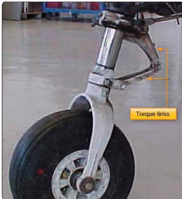
Figure 6.19 – Torque links align the landing gear and retain the piston in the upper cylinder when the strut is extended
