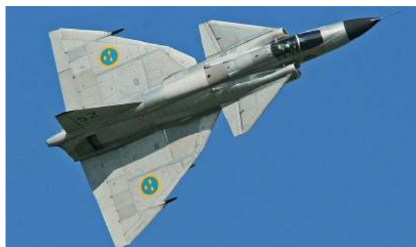
Figure 4.4 – A Saab 37 Viggen, the first modern canard aircraft to go into production
