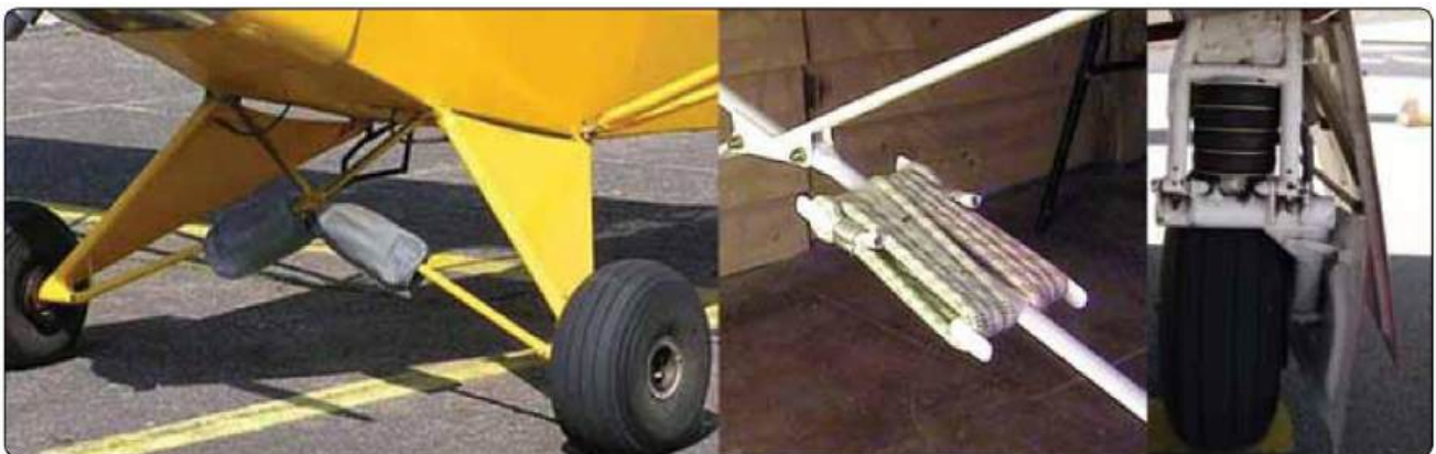
Figure 6.15 – Piper Cub bungee cord landing gear transfer landing loads to the airframe (left and center). Rubber, donut-type shock transfer is used on some Mooney aircraft (right)
