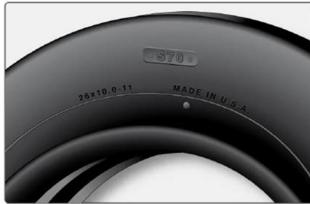
Figure 6.37 – A sidewall vent marked by a colored dot must be kept free from obstruction to allow trapped air or nitrogen to escape from the carcass plies of the tire
