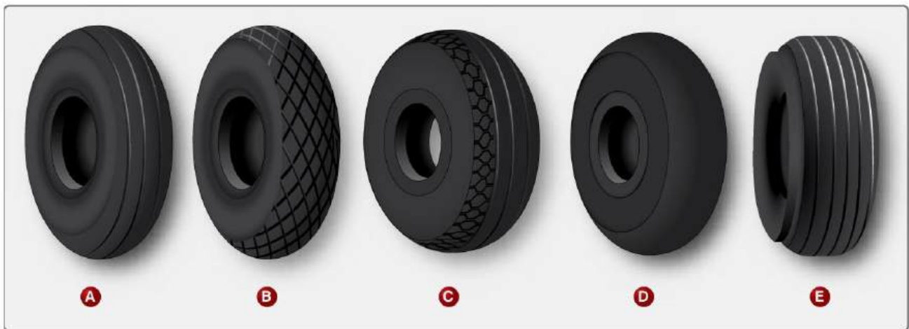
Figure 6.36 – Aircraft tire treads are designed for different uses. A is a rib tread designed for use on paved surfaces. It is the most common aircraft tire tread design. B is a diamond tread designed for unpaved runways. C is an all-weather tread that combines a ribbed center tread with a diamond tread pattern of the edges. D is a smooth tread tire found on older, slow aircraft without brakes designed for stopping. E is a chine tire used on the nose gear of aircraft with fuselage mounted jet engines to deflect runway water away from the engine intake(s)
