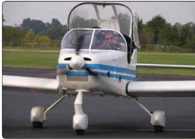
Figure 6.13 – Non-shock absorbing struts made from steel, aluminum, or composite material transfer the impact forces of landing to the airframe at a non-damaging rate
