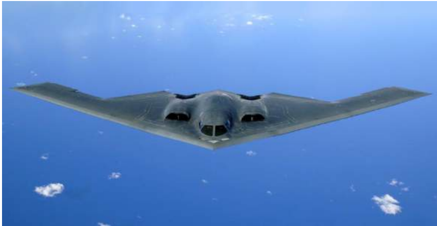
Figure 4.1 – B-2 Spirit (the Stealth Bomber) it is a flying wing design with a crew of two
