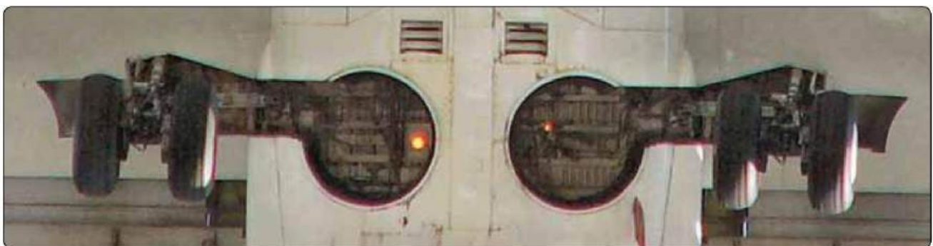
Figure 6.12 – The retractable gear of a Boeing 737 fair into recesses in the fuselage. Panels attached to the landing gear provide smooth airflow over the struts. The wheel assemblies mate with seals to provide aerodynamic flow without doors
