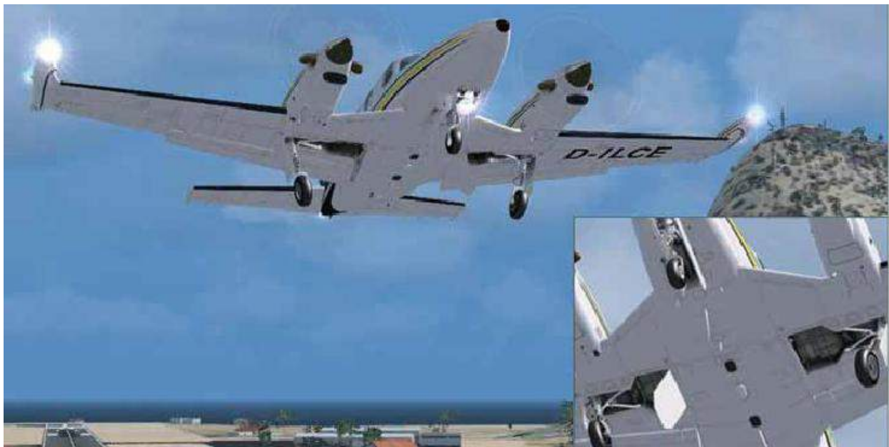
Figure 3.18 – Wheel wells in a wing engine nacelle with gear coming down (inset)
