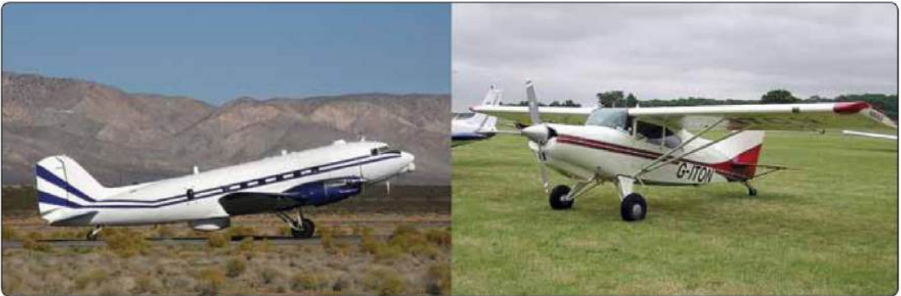
Figure 6.3 – Tail wheel configuration landing gear on a DC-3 (left) and a STOL Maule MX-7-235 Super Rocket
