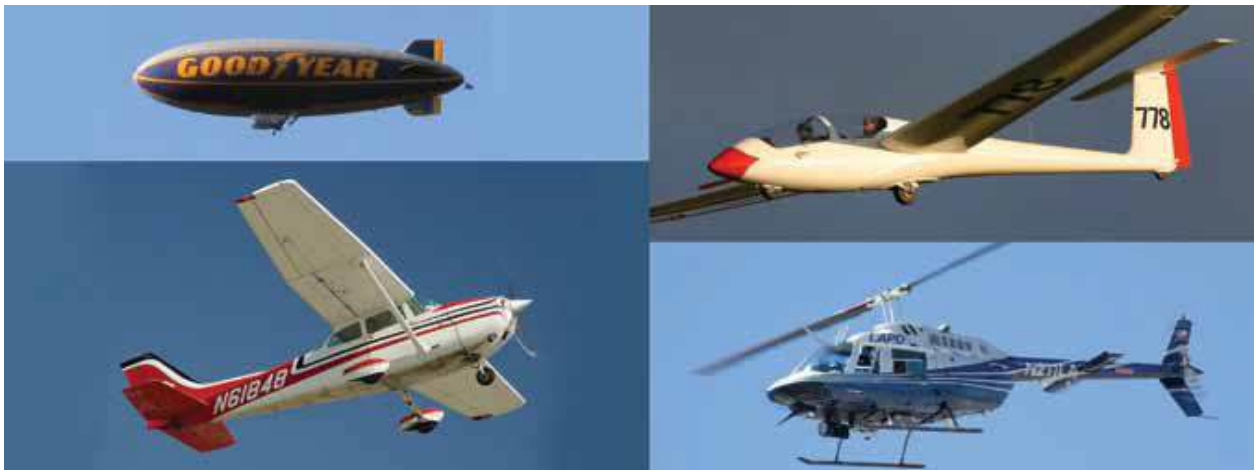
Figure 2.1 – Examples of different categories of aircraft, clockwise from top left: lighter-than-air, glider, rotorcraft, and airplane.
