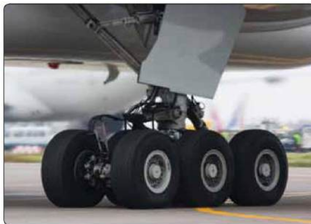
Figure 6.9 – Triple bogie main landing gear assembly on a Boeing 777
