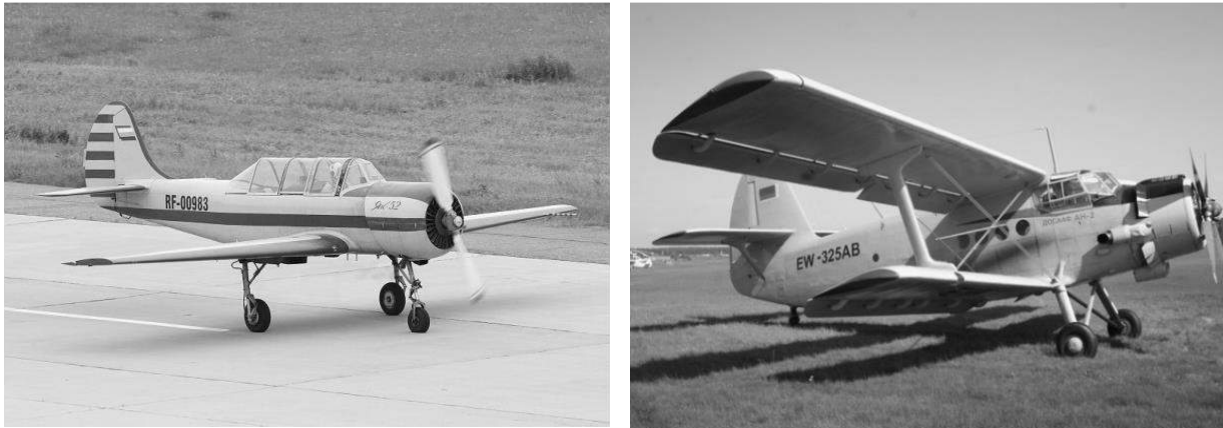
Fig. 4.4. Airplanes: a monoplane and a biplane
