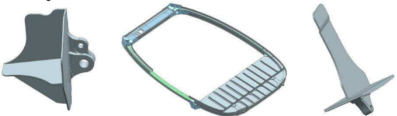
Fig. 5.19. Analytical Standards of Landing Gear Attachment Fitting and Assembly Model of Strong Frame
