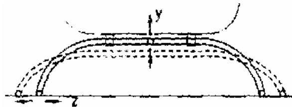
Fig. 3.32. Spring Deformation of Skid Landing Gear during Landing
