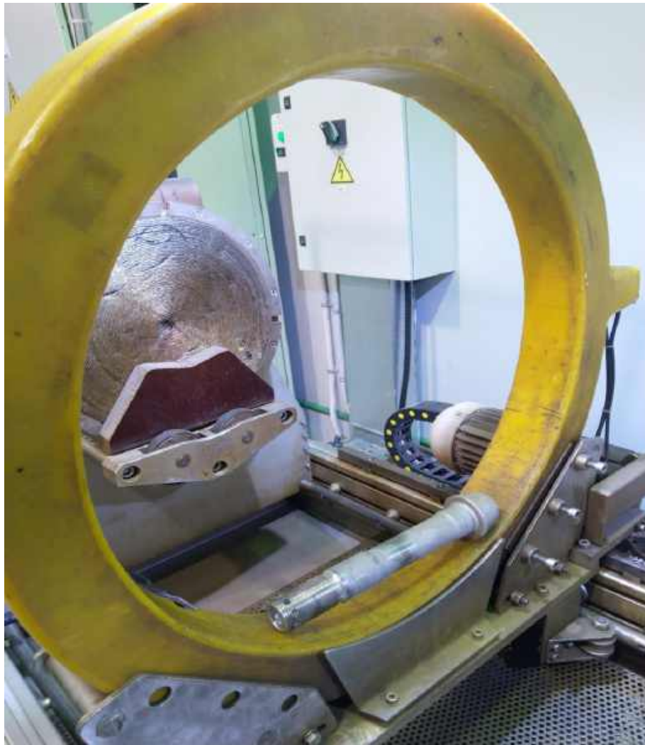
Figure 3.6 – Bolt's placement in the machine's solenoid
