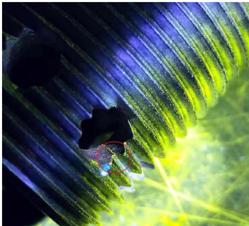
Figure 3.14 – Crack in the wall of the countersink hole.
