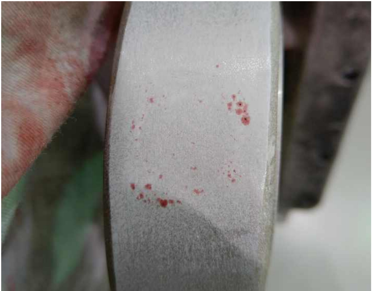
Figure 4.11 – Pores in the material of the Mi-8 vibration damper
