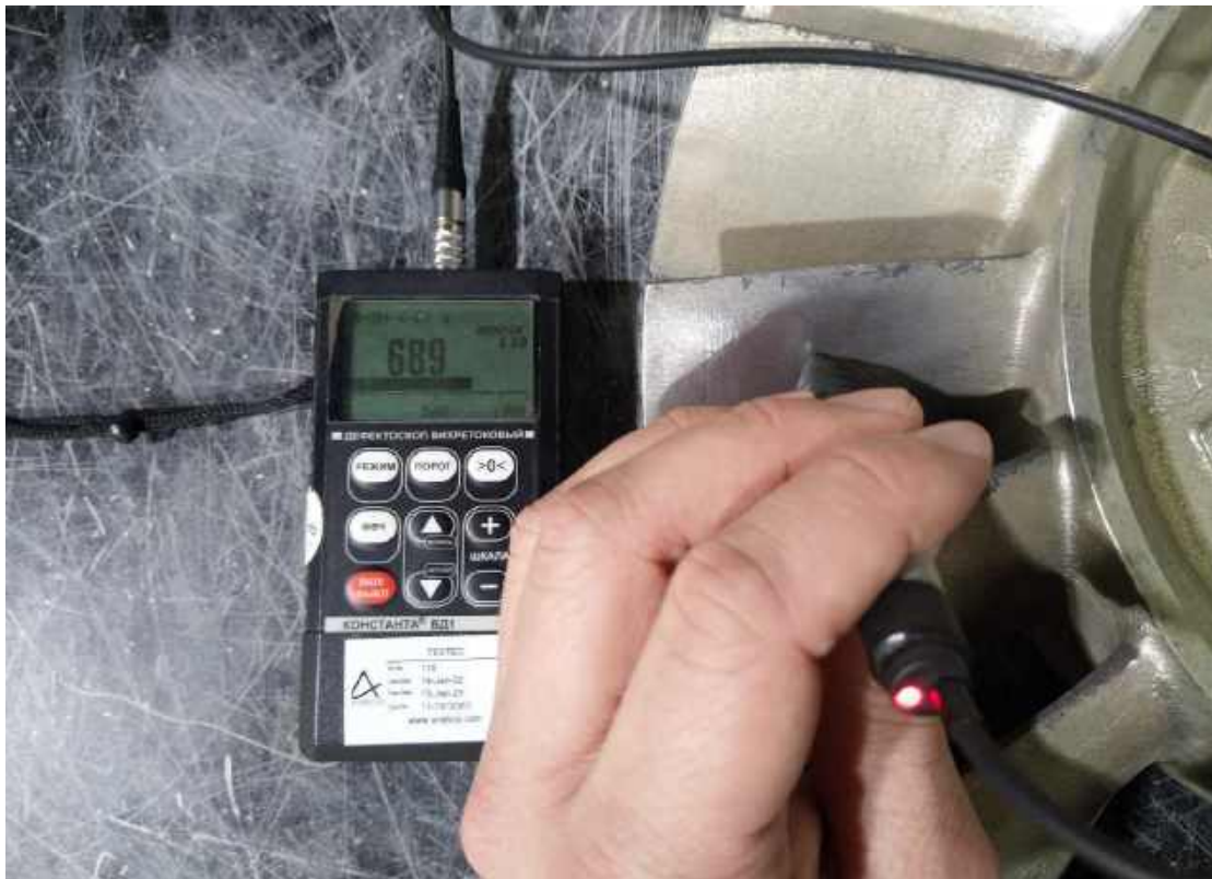
Figure 5.10 – The defect 689 \mu\text{m} depth found during eddy-current testing
