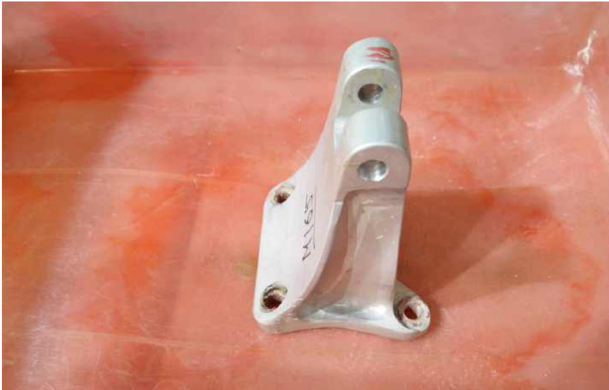
Figure 4.4 – Cleaned and dried fuel tank mounting bracket in the inspection zone
