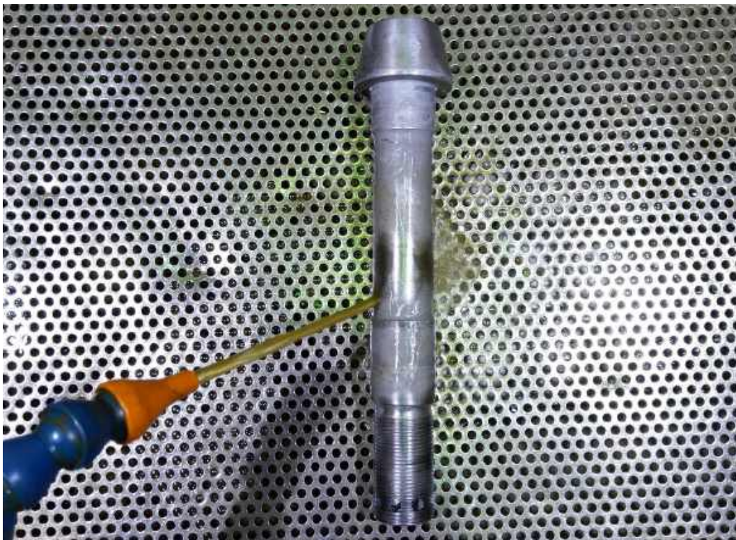
Figure 3.8 – Suspension is not the only form of particles that can be applied to the part – magnetic particles are also exist in form of dry or wet powder
