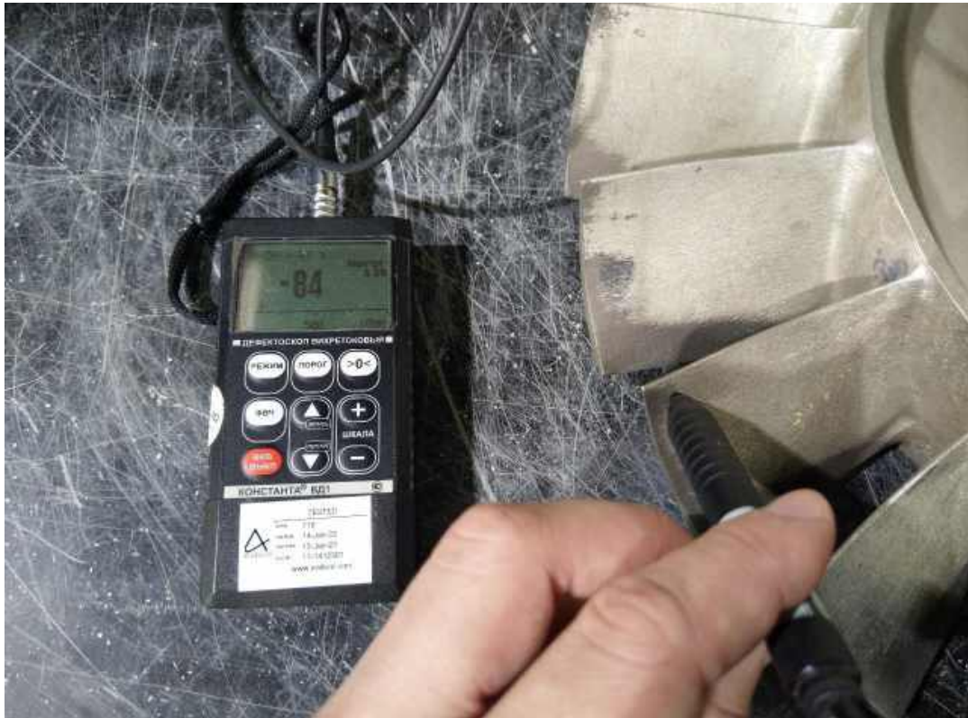
Figure 5.8 – The beginning of eddy-current testing of the blower wheel; the value on the display is negative because the current surface height is bigger than the height of the surface which was used to configure the flaw detector
