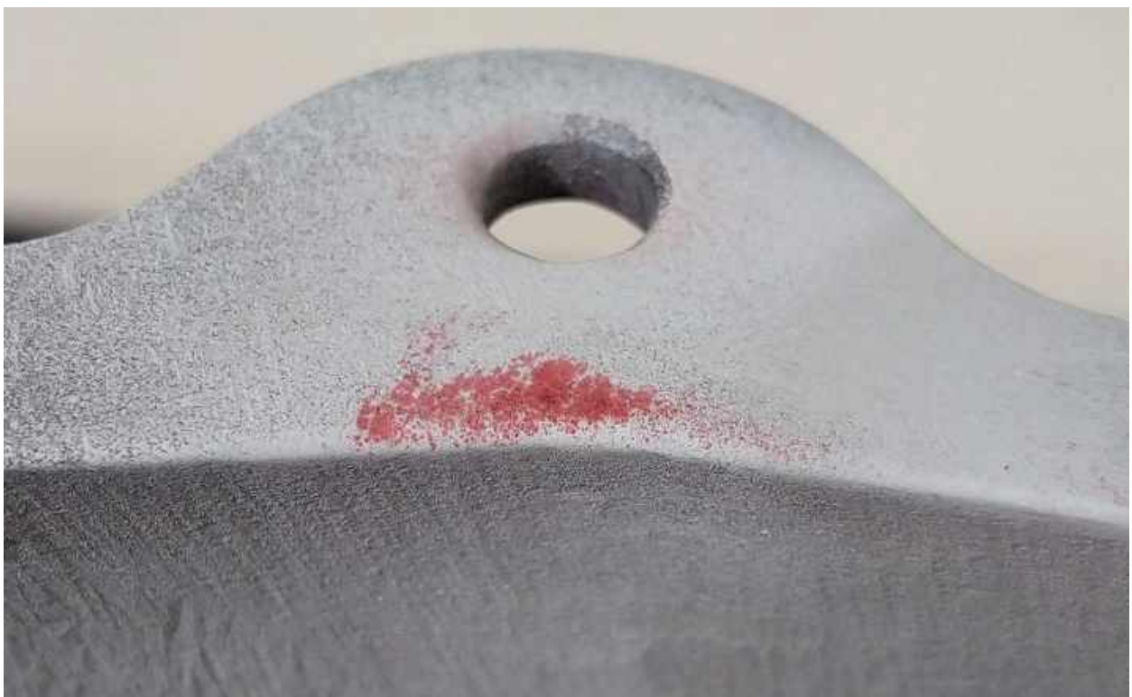
Figure 4.12 – Fatigue cracks in the Mi-8 blower
