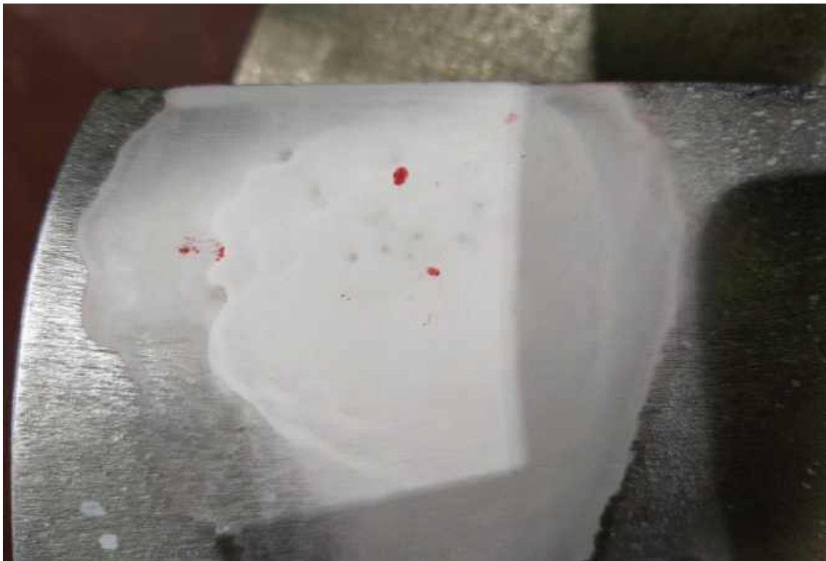
Figure 5.13 – Liquid penetrant testing results
