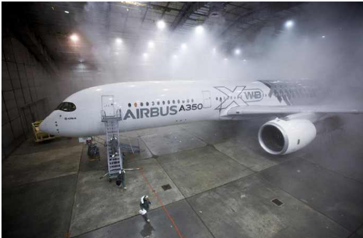
Figure 6 – Airbus A350 XWB undergoing two weeks of testing at the McKinley Climate Laboratory in Florida, USA
