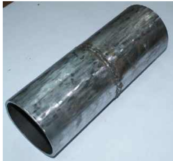
Figure 6.4 – A sample of pipe welding connection
