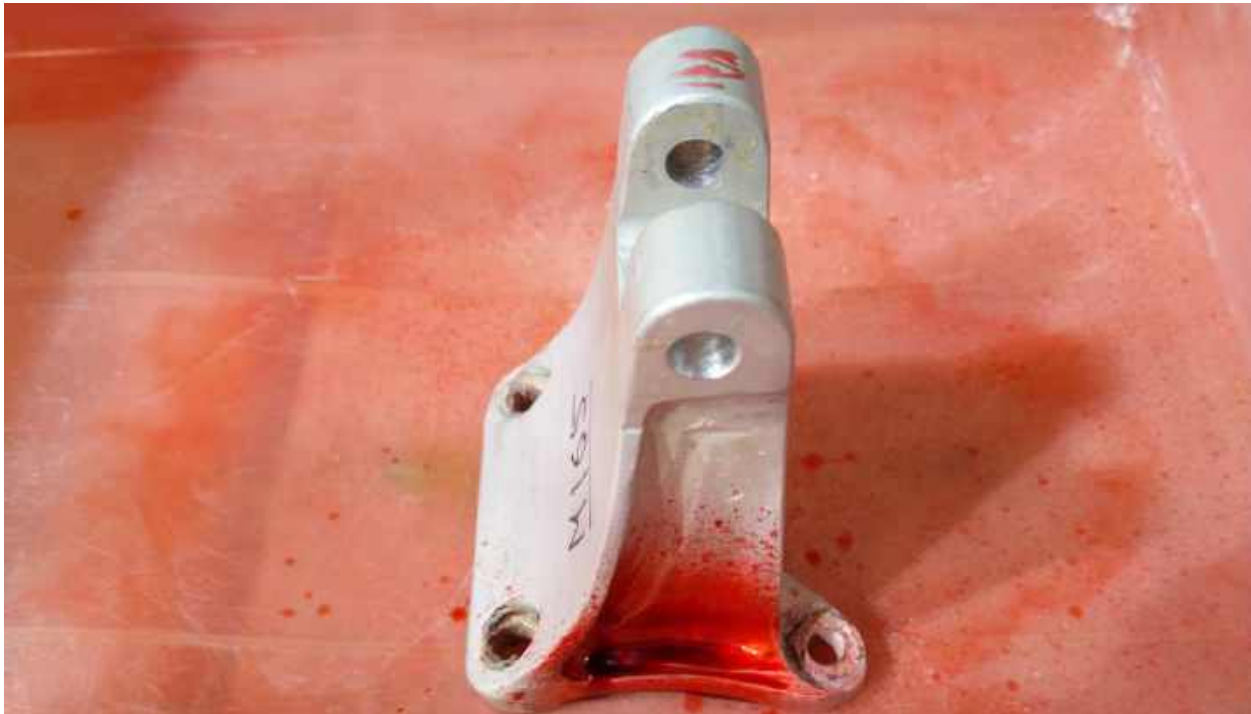
Figure 4.5 – Fuel tank mounting bracket covered with penetrant
