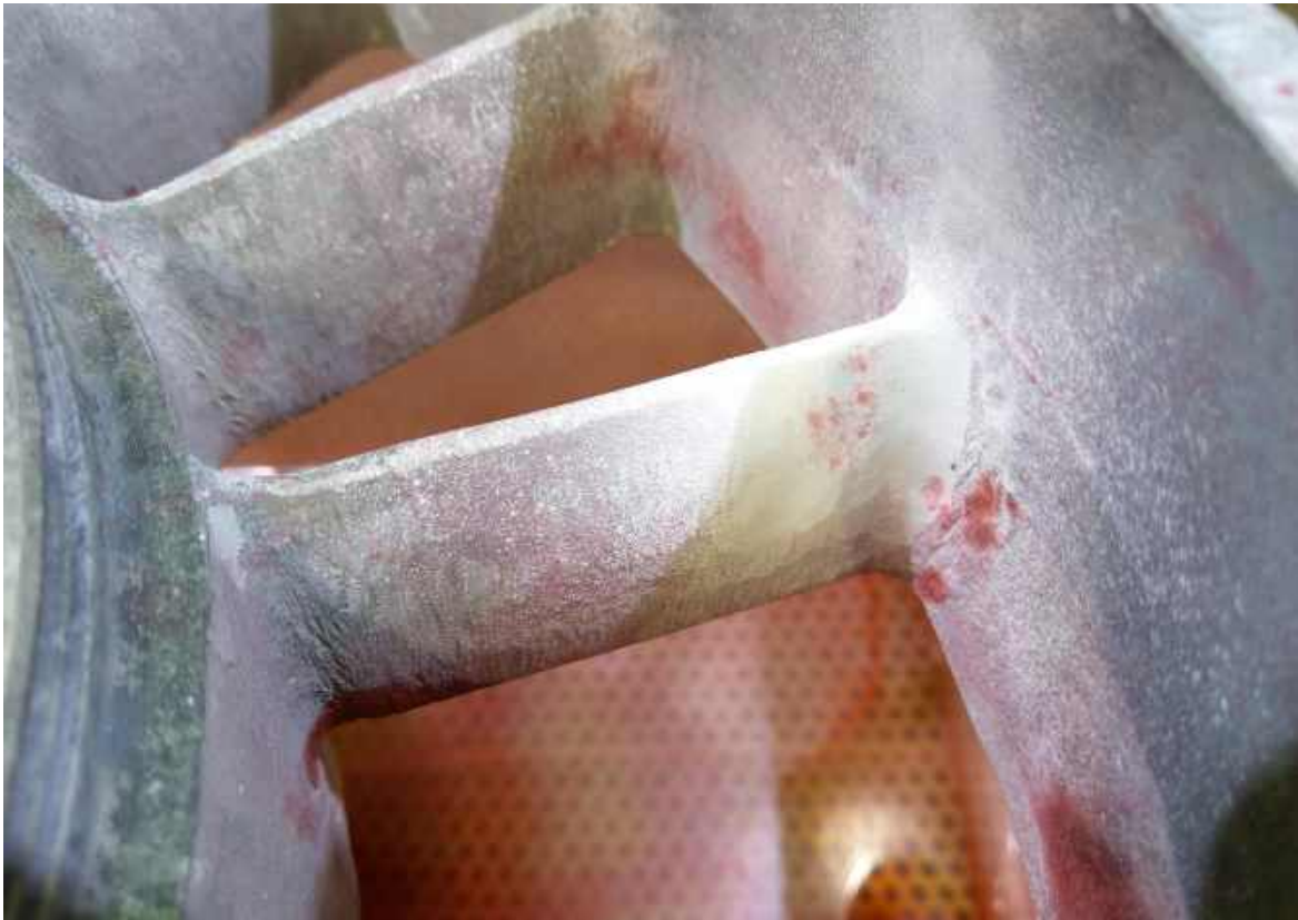
Figure 4.9 – Corrosion on the blades of the Mi-8 blower
