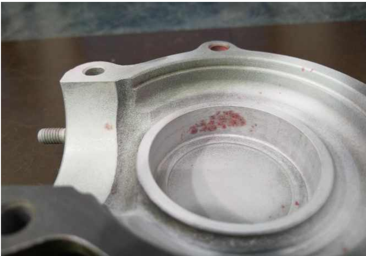
Figure 4.10 – Corrosion on the Mi-8 air compressor
