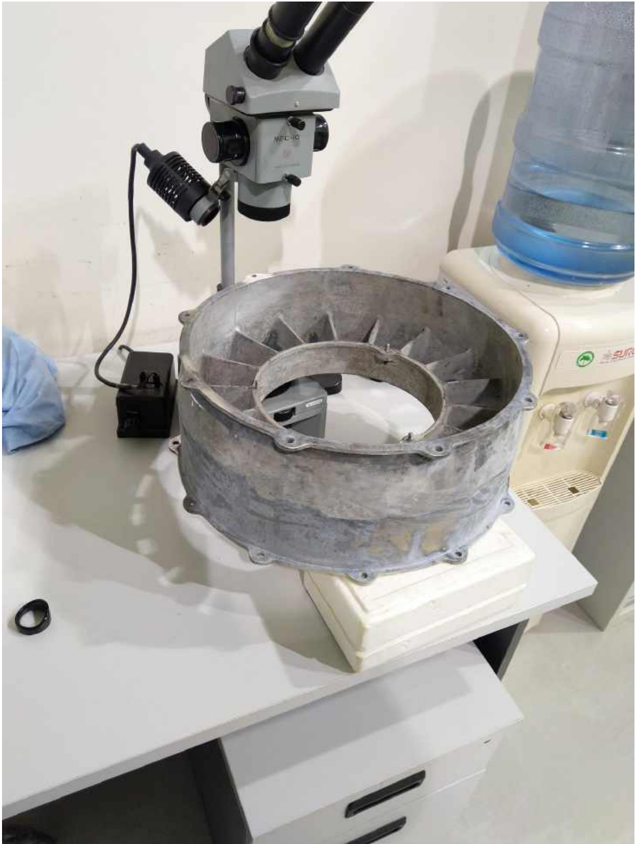
Figure 5.14 – Guiding devise of the blower; the microscope is pointed at the area where the defects were found to confirm their presence visually
