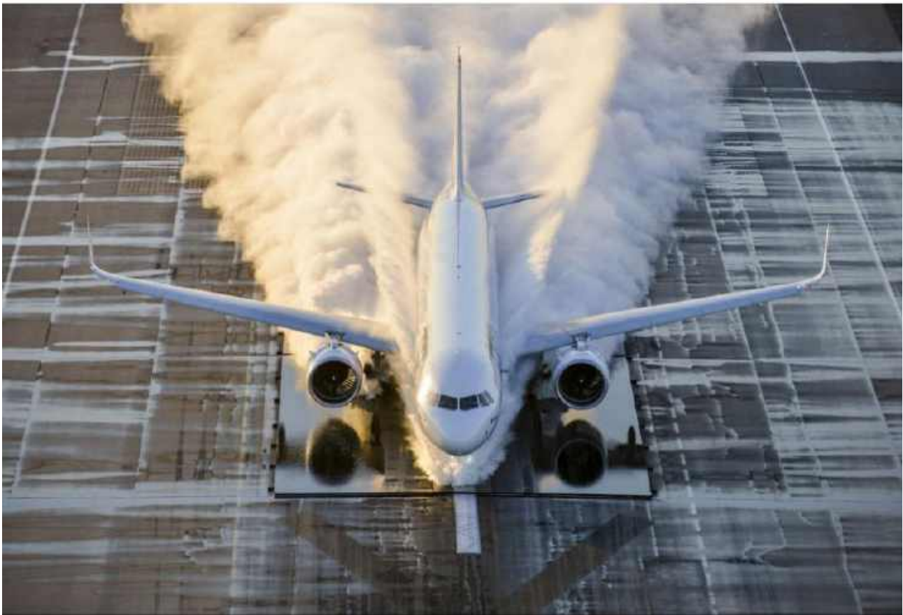
Figure 4 – The Airbus A321neo has undergone a water impact test as part of its certification campaign
