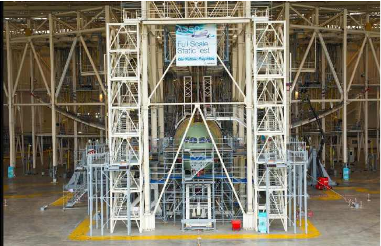
Figure 5 – A350 XWB wings tested at ultimate load, showing wing tip deflection of five meters
