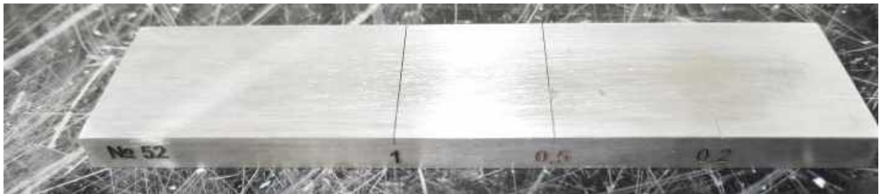
Figure 5.5 – Specimen with artificially created cracks with a depth of 1, 0.5 and 0.2 mm
