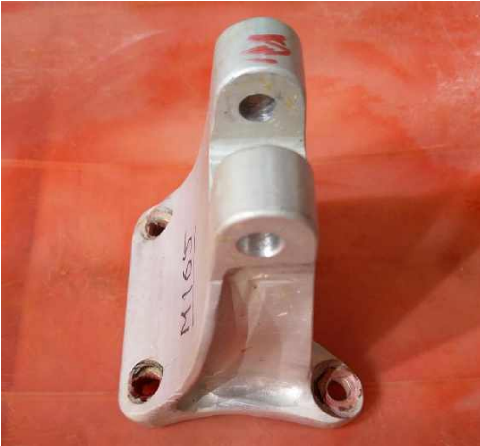
Figure 4.6 – Fuel tank mounting bracket after penetrant removal and drying
