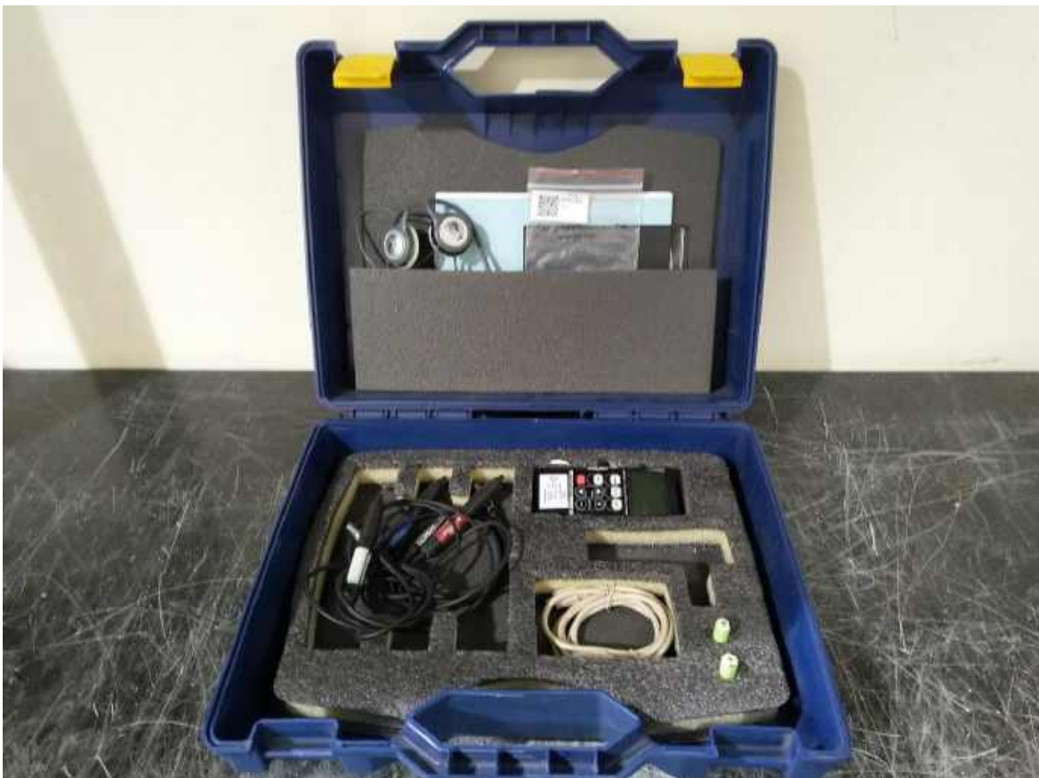
Figure 5.3 – Konstanta VD-1 flaw detector with set of probes for different materials
