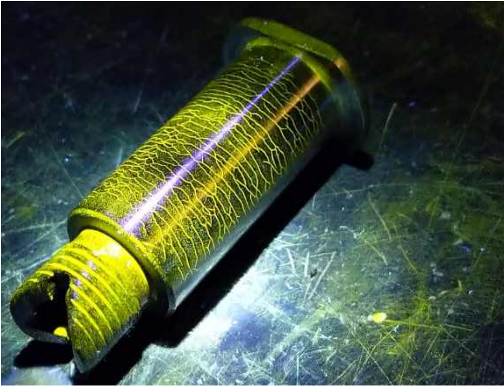
Figure 3.17 – Detection of cracks formed during grinding using magnetic particle testing
