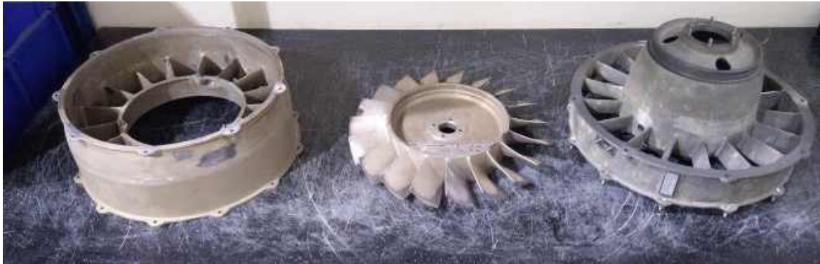
Figure 5.2 – Parts of the blower tested with eddy-current method
