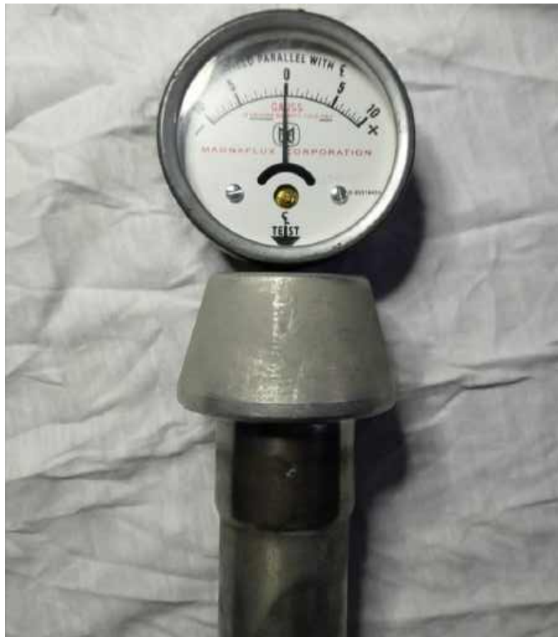
Figure 3.15 – Position of the instrument arrow at the demagnetized part
