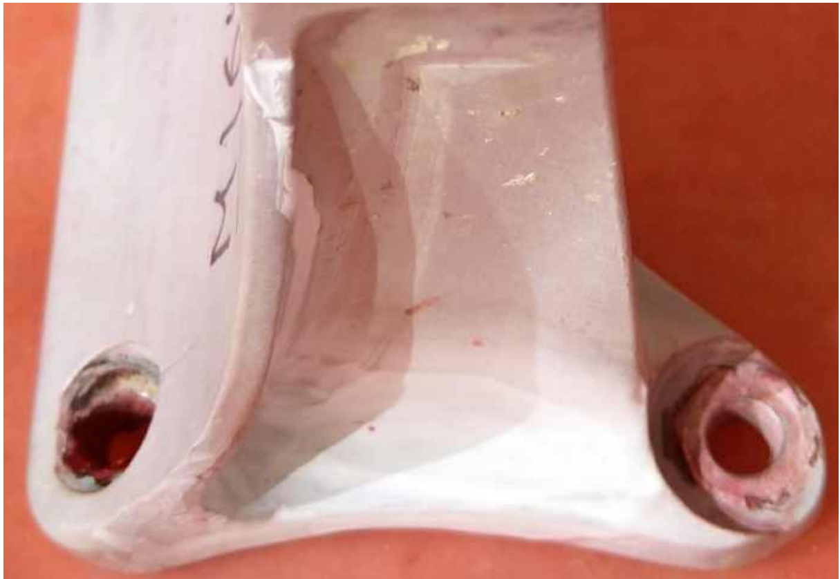
Figure 4.7 – Area of the fuel tank mounting bracket covered with white developer
