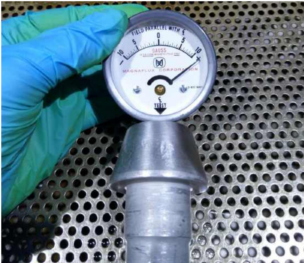
Figure 3.7 – Arrow on the instrument shows how strongly the part is magnetized
