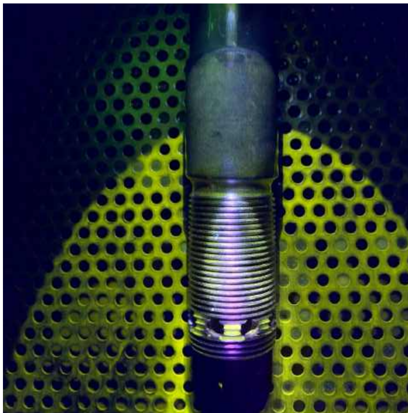
Figure 3.10 – Mounting bolt covered with magnetic particles (yellow) under ultraviolet light
