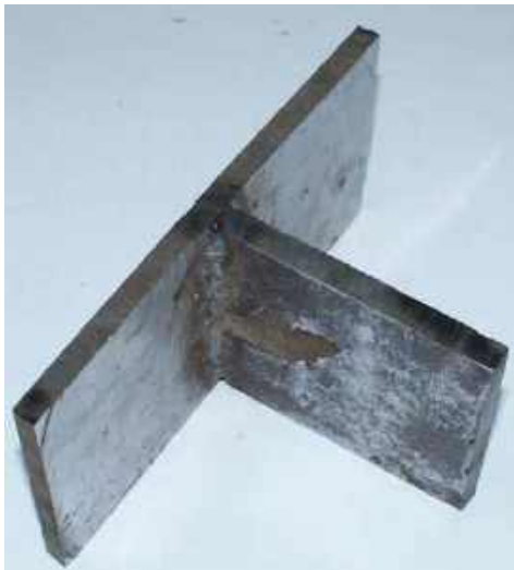
Figure 6.3 – A sample of a welded joint
