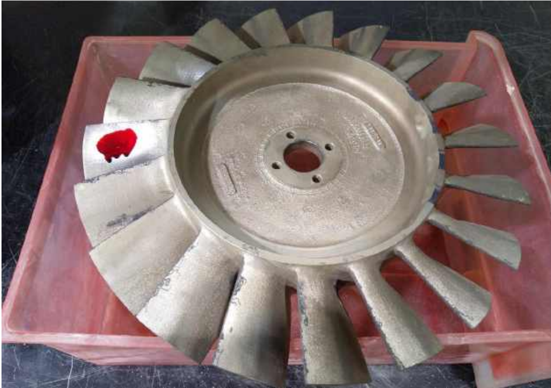
Figure 5.12 – One of the steps of liquid penetrant testing of the blower wheel
