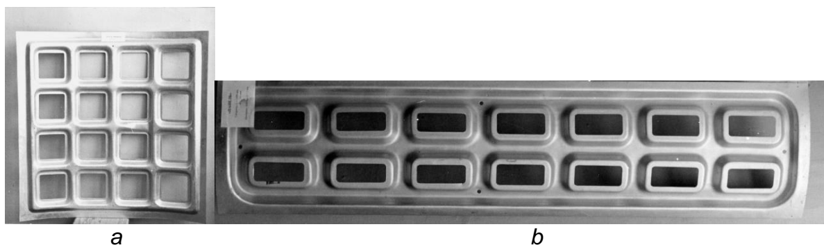
Fig. 8. Panels of rigidity pressed by ПЭГ-ХАИ-500:
