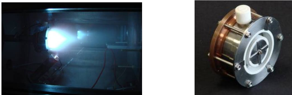
Fig. 4. PPI thruster and run in the vacuum chamber of the laboratory GREMI
