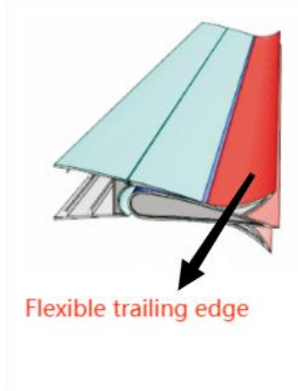
Figure 1.21 — Flexible trailing edge section
