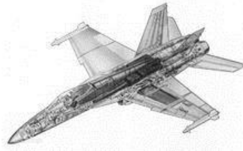
Figure 1.5 — General layout breakdown of F/A-18 combat attack aircraft
