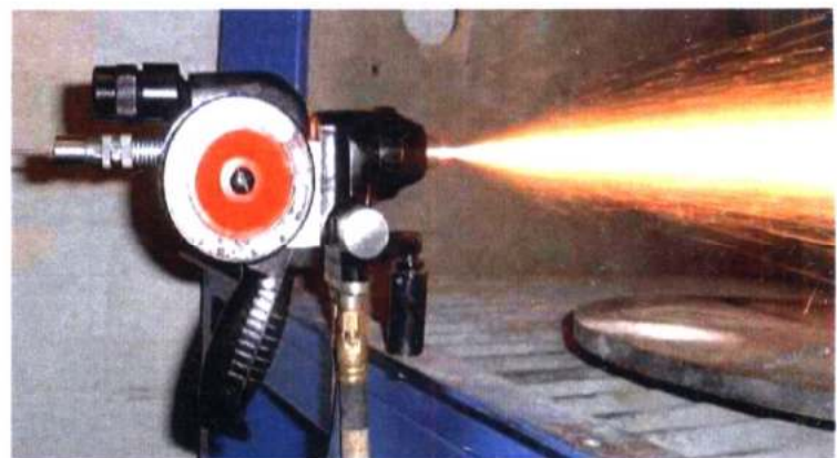
Fig.1.6. Recent Gun Spraying 13% Chromium Steel (Source: Metco Ltd. )
