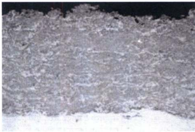
Fig.1.13. HVOF Sprayed Tungsten Carbide/12% Cobalt Coating [8]
