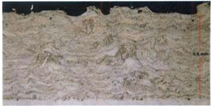
Fig.1.16. Arc Wire Sprayed 13Cr Steel Coating (Source: Gordon England)
