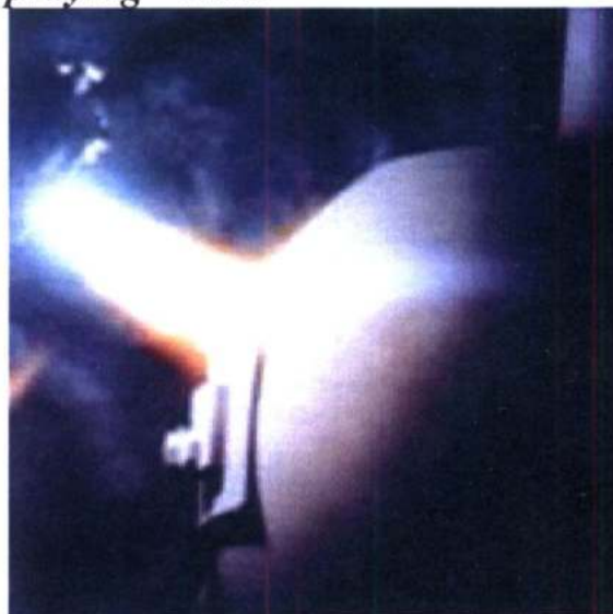
Fig.1.21. The Atmospheric Plasma Spraying Process (Source: AP&C Advanced Powders & Coatings Inc.)
