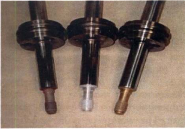
Fig.1.40. Shows the damper piston thread before plating, after cadmium and after the Type II coating ( Source: Brooktronics Engineering Corporation )
