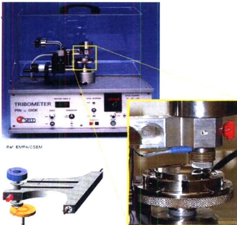
Fig.5.9. The Wear Testing Machine (Source: EMPA)
