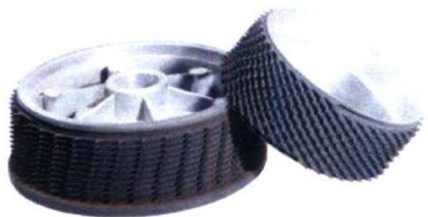
Fig.3.17. Texturizing Rings (Source: Plasma & Thermal Coatings Ltd.)
