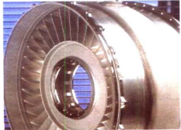
Fig.3.2. RB199 Multivane with Abradable coating for clearance control (Source: Plasma & Thermal Coatings Ltd.)
