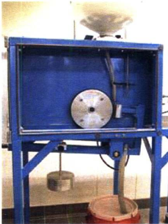
Fig.5.3. Abrasion testing machine (Source: EMPA)
