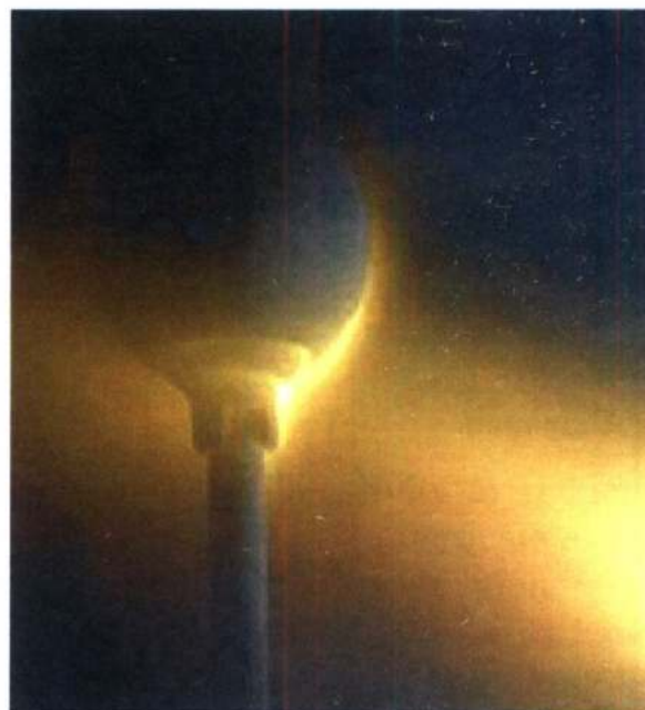
Fig.1.22. The Vacuum Plasma Spraying Process (Source: AP&C Advanced Powders & Coatings Inc.)
