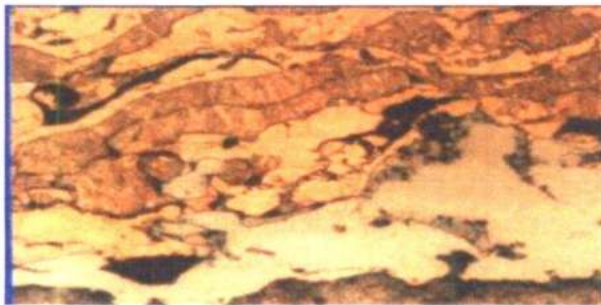
Fig.1.8. Combustion Powder Sprayed Copper Aluminium Composite (aluminium bronze ) Coating (Source: Gordon England)
