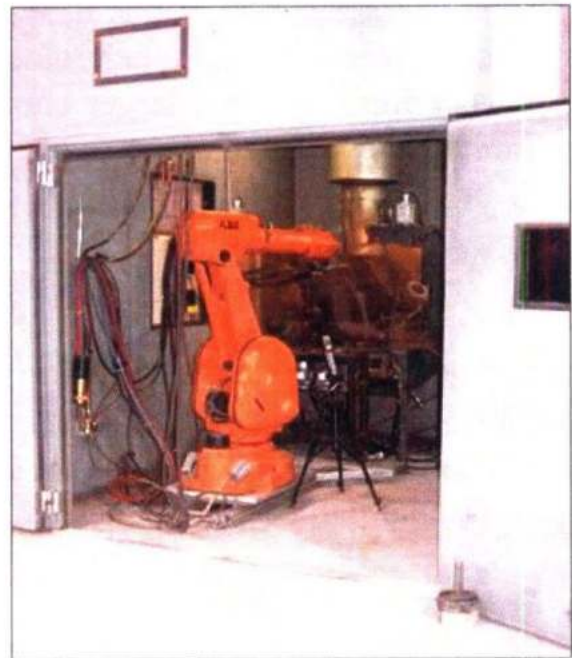
Fig.1.11. The HVOF Process Robot (Source: AP&C Advanced Powders & Coatings Inc.)
