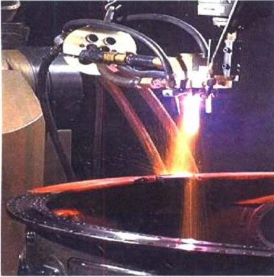
Fig.1.18. The Plasma Spraying Process (Source: Plasma Group Science)
