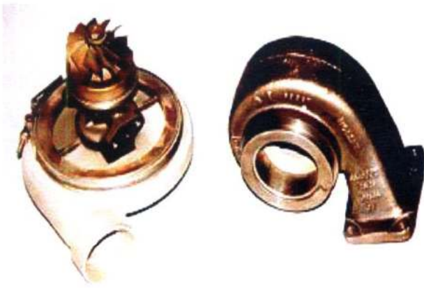
Fig.3.4. TurboCharges with abrasion resistant coatings (Source: Plasma & Thermal Coatings Ltd.)
