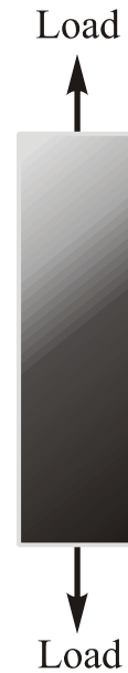
Fig. 2.16 Slip bands (or a Luders' bands) in a polished steel specimen loaded in tension
