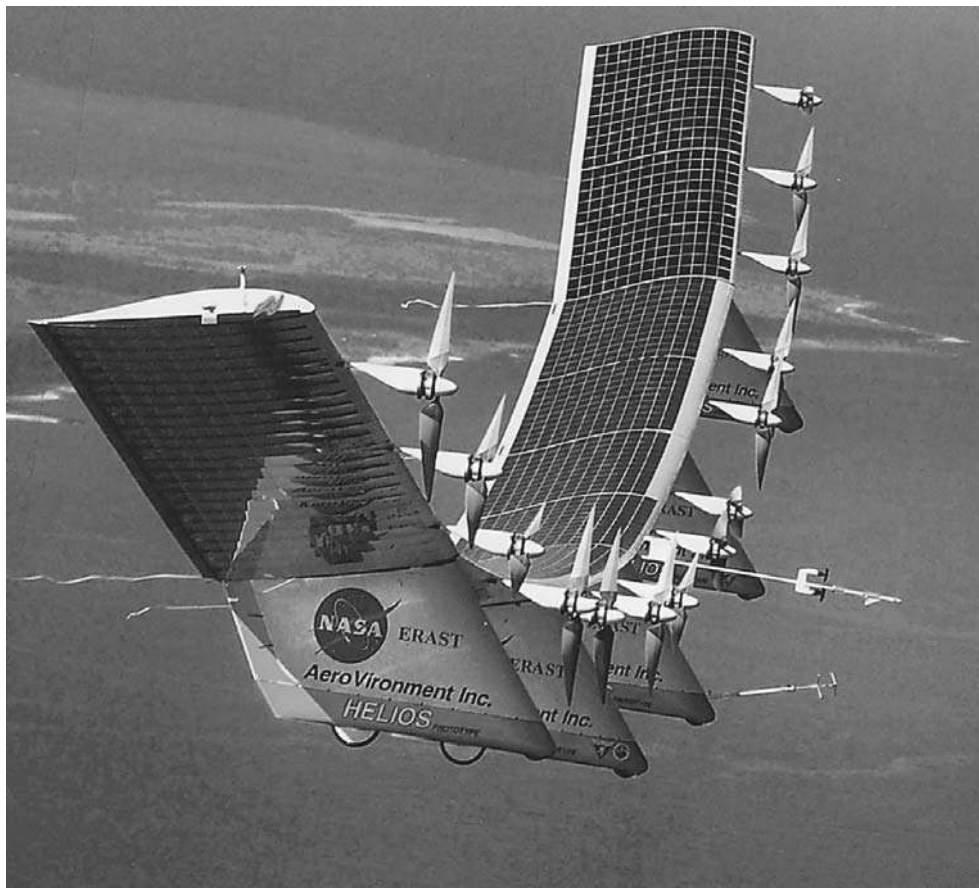
Fig. 11.13. «Helios» Large-Scale Unmanned Experimental Aircraft with the Propulsion System Composed of Electric Motors Powered by Solar Batteries
