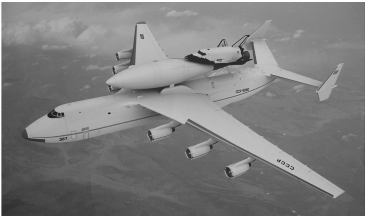
Fig. 11.7. Earth-to-Orbit Vehicle Launching by An-225 Mriya Super-Heavy Cargo Aircraft (project)
