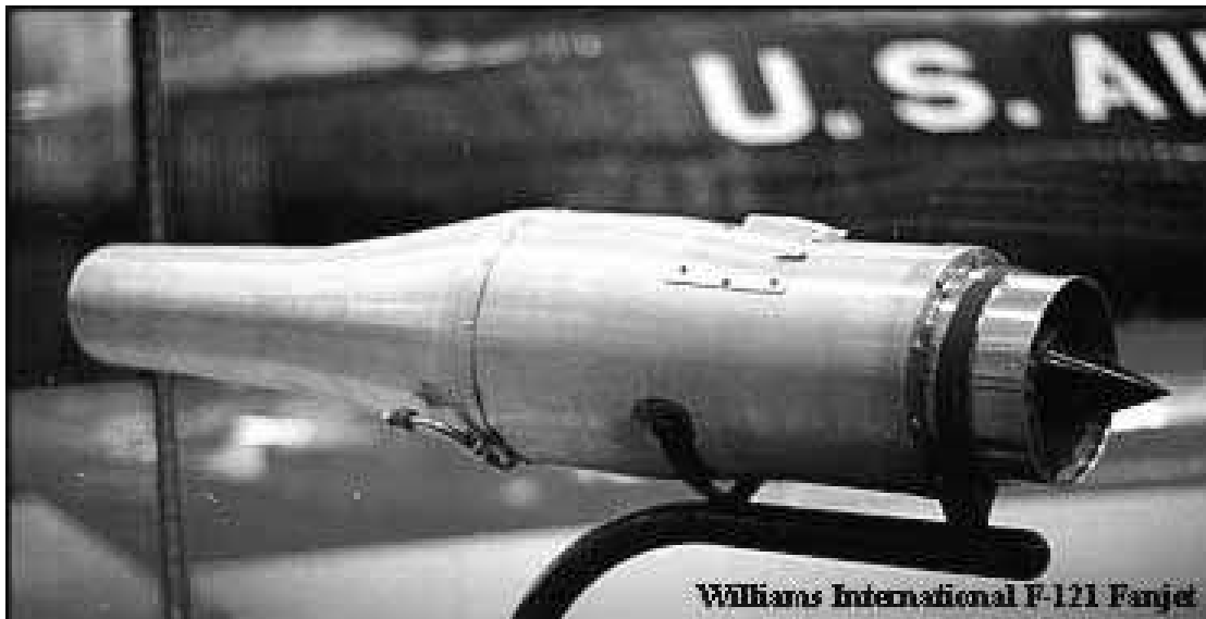
Fig. 11.38. AGM-136 Anti-Radar Missile (a) and its By-Pass Turbojet F-121 (b)
