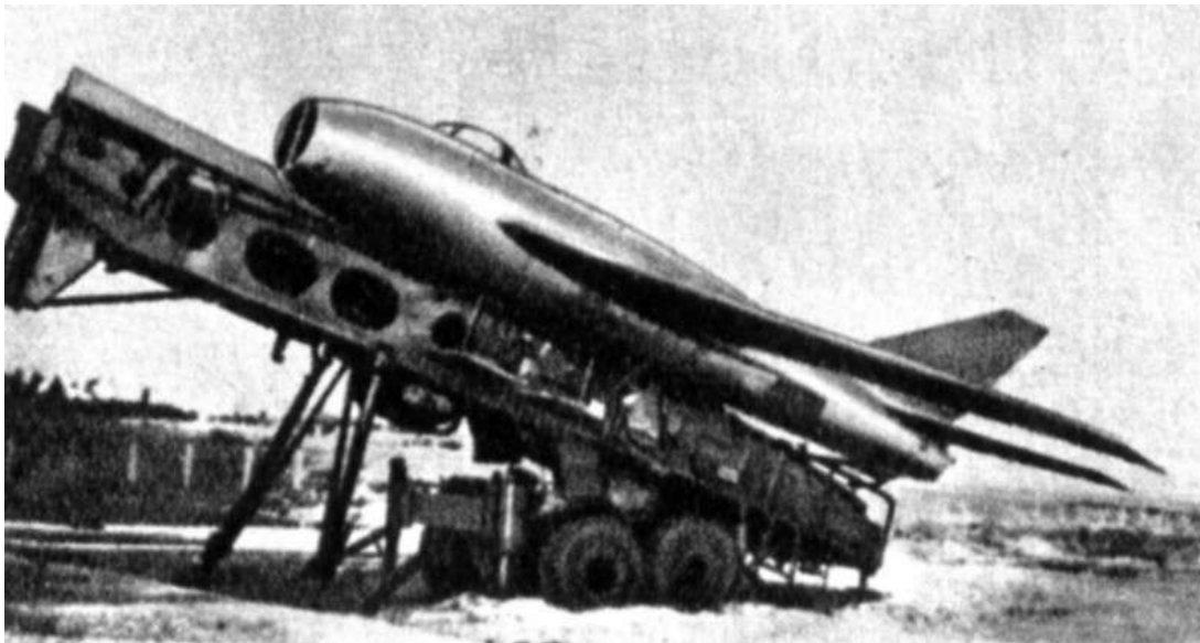
Fig. 11.46. Fighter With Powerful Solid-Propellant Booster Rockets on Short Launcher Rails Mounted on Truck Trailer
