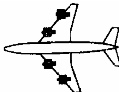
Fig. 2.33. Arrangement of (Bypass) Turbojets under Wing with Pylons
