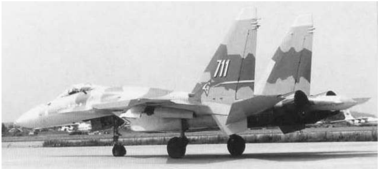
Fig. 11.27. Su-37 Fighter Power Plant with Deflectable Thrust Vector
