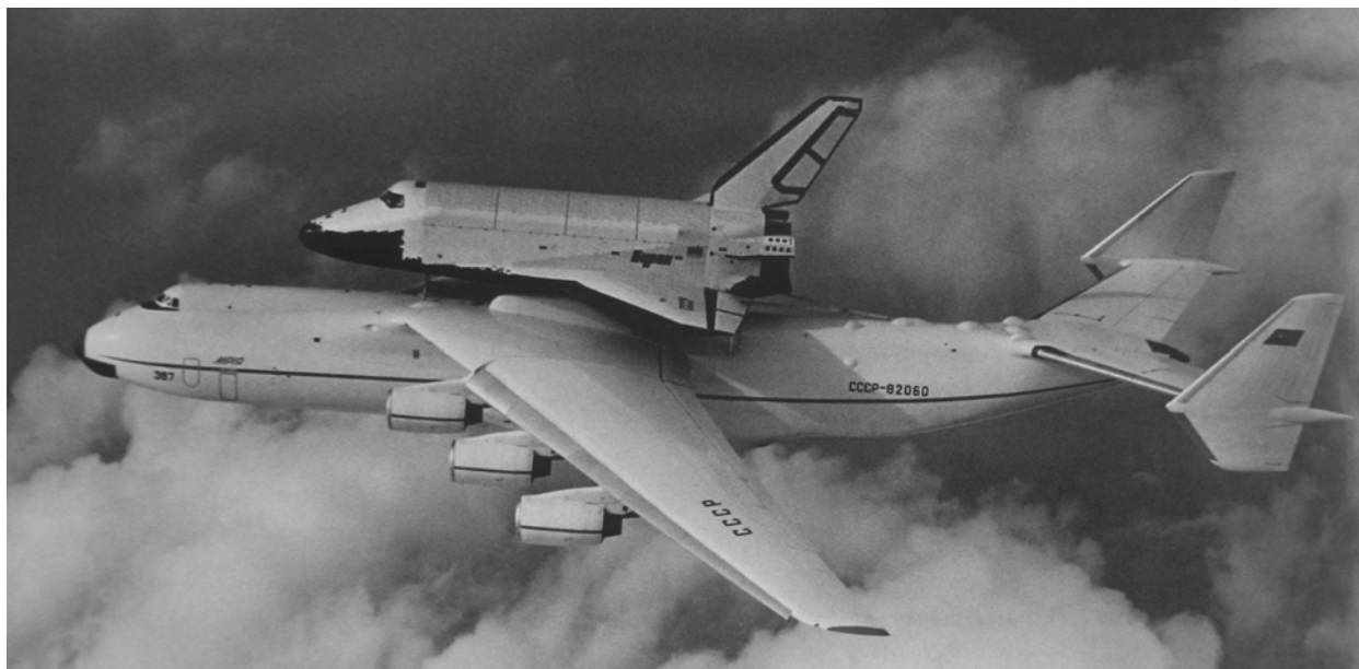
Fig. 11.5. Transportation of Soviet Буран Aerospace Aircraft as External Load Fastened to the Fuselage of the An-225 Мрія
